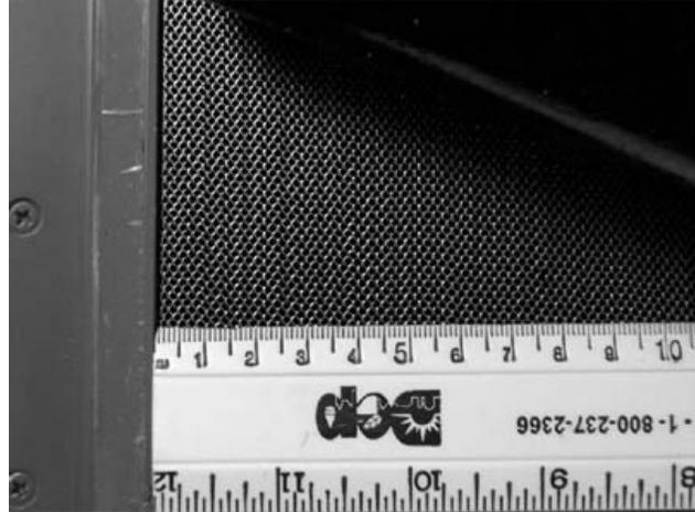
Figure 1-11. Back of Collimator Showing Corrugated Lead Strips
