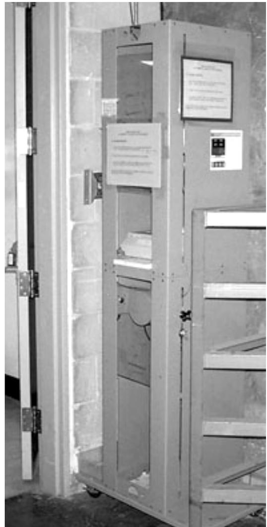
Figure 1-16. Detector Assembly of the HMC Waste Monitor
