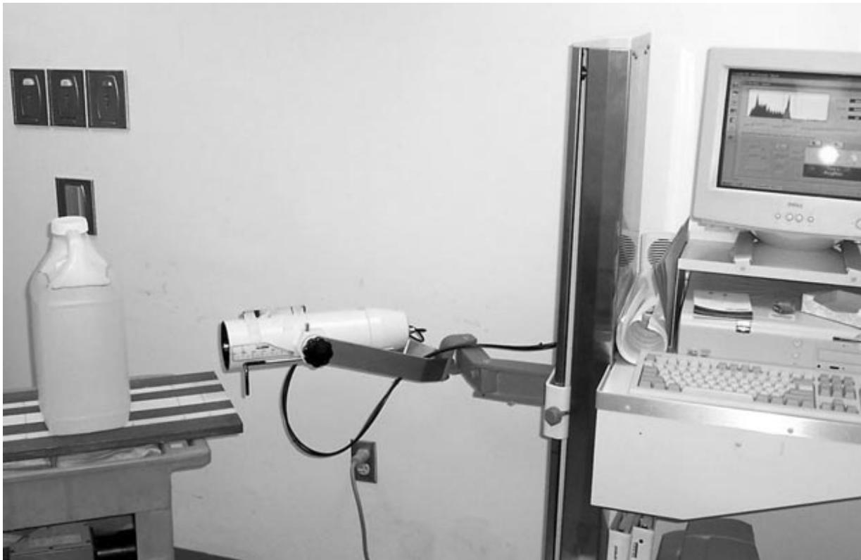
Figure 1-13. Atomlab 950 Thyroid Uptake System
