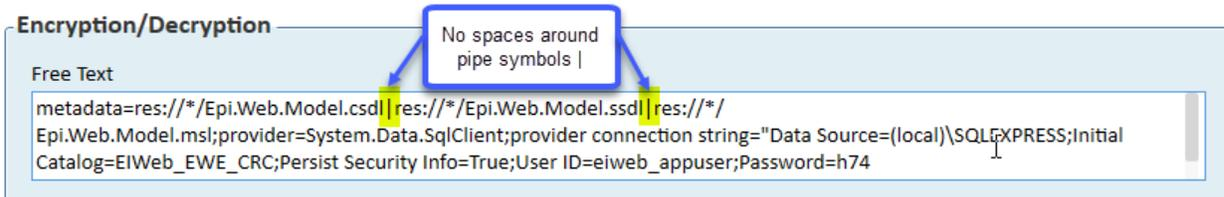
Figure 15: Ensure no extra spaces are added when copying from a PDF.
