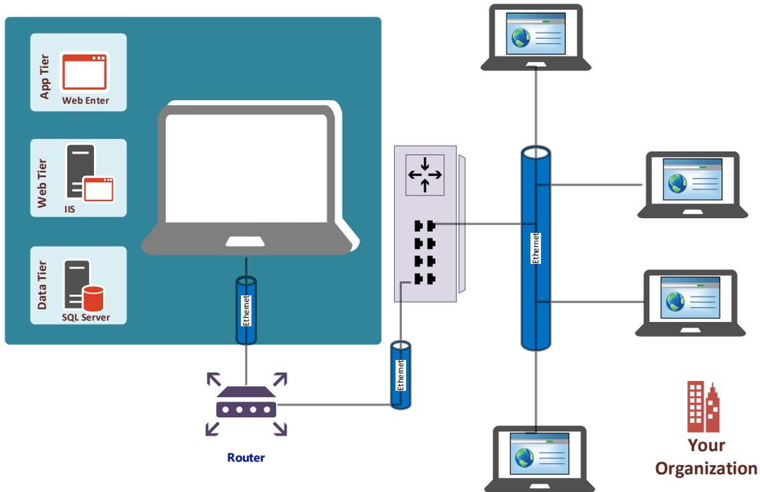
Figure 3: CRC eTool in wired network configuration
