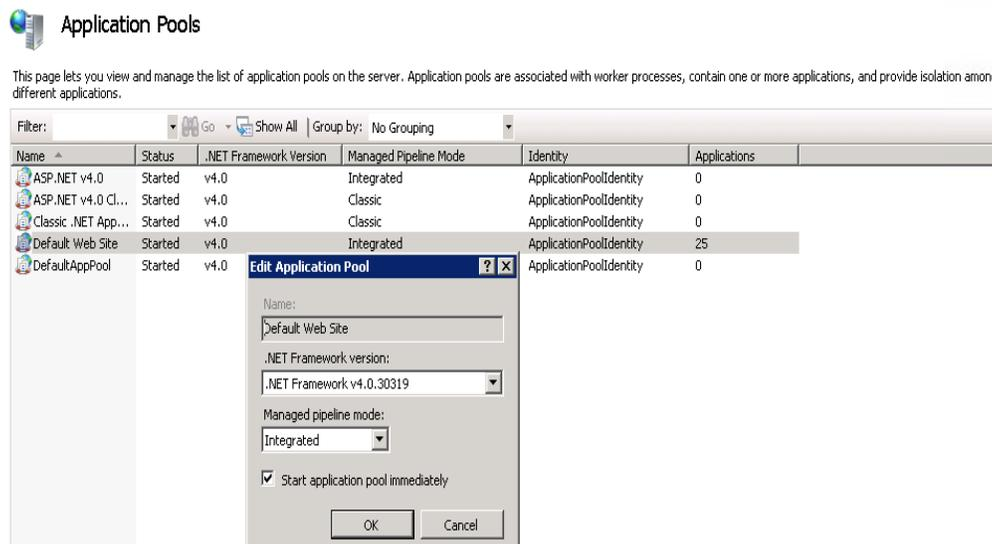
Figure 8: Application pool configured using .NET 4.0
