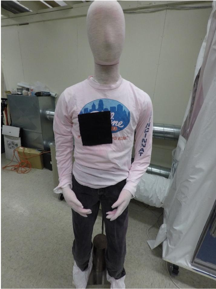
Figure 3. Research manikin showing placement of fabric swatch on the shirt. (Photo credit: NIOSH)
