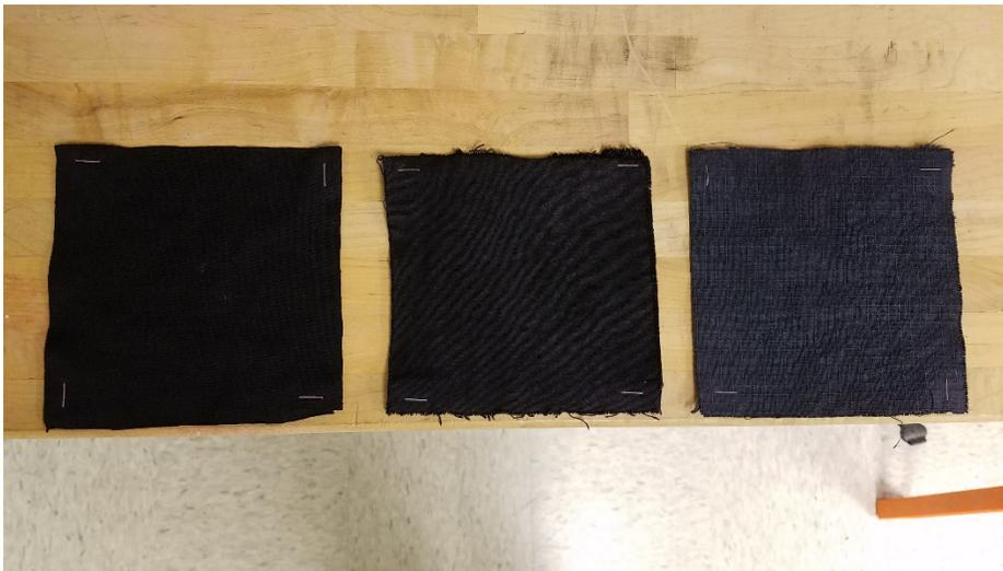
Figure 11. Swatches of the three different fabrics used in experiments. From left to right, polyester double-knit (DK), cotton denim (DM) and firefighter turnout fabric (FF). Staples in the four corners of each swatch hold small squares of Velcro in place. (Photo credit: NIOSH)
