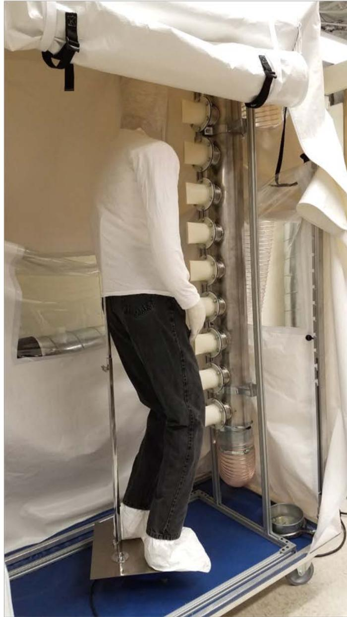
Figure 2. Manikin standing on turntable inside of chamber; one of the nozzle manifolds is visible with one side of the chamber opened. (Photo credit: NIOSH)
