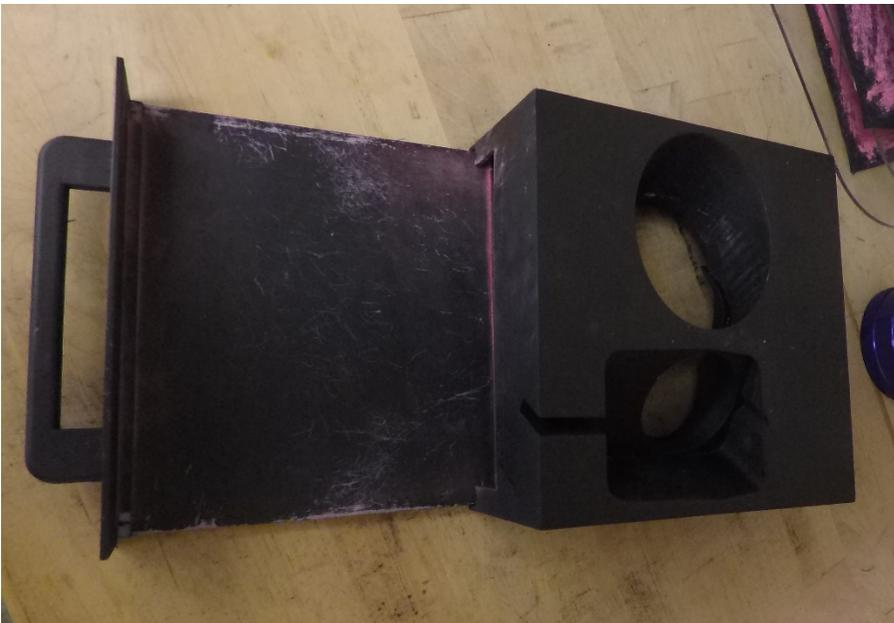
Figure 9. Support used for measuring the fluorescence of a fabric swatch. The swatch is placed in the open drawer at left and slid inside the support. (Photo credit: NIOSH)
