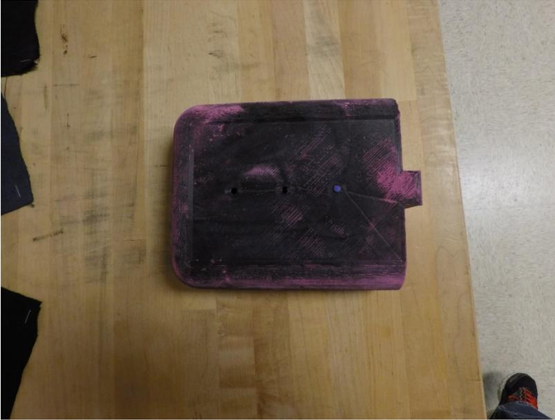
Figure 8. The bottom of the 3-D application chamber, showing the blue pin that deflects and scatters injected model soil. (Photo credit: NIOSH)
