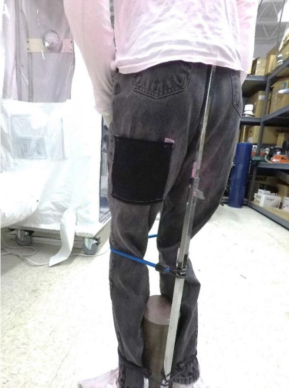
Figure 4. Research manikin showing placement of fabric swatch on the leg. (Photo credit: NIOSH)
