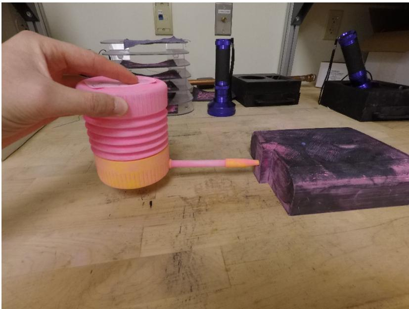
Figure 7. Method of applying model soil to a fabric swatch, using a pesticide duster and a 3-D printed application chamber. The fabric is placed beneath the chamber. (Photo credit: NIOSH)
