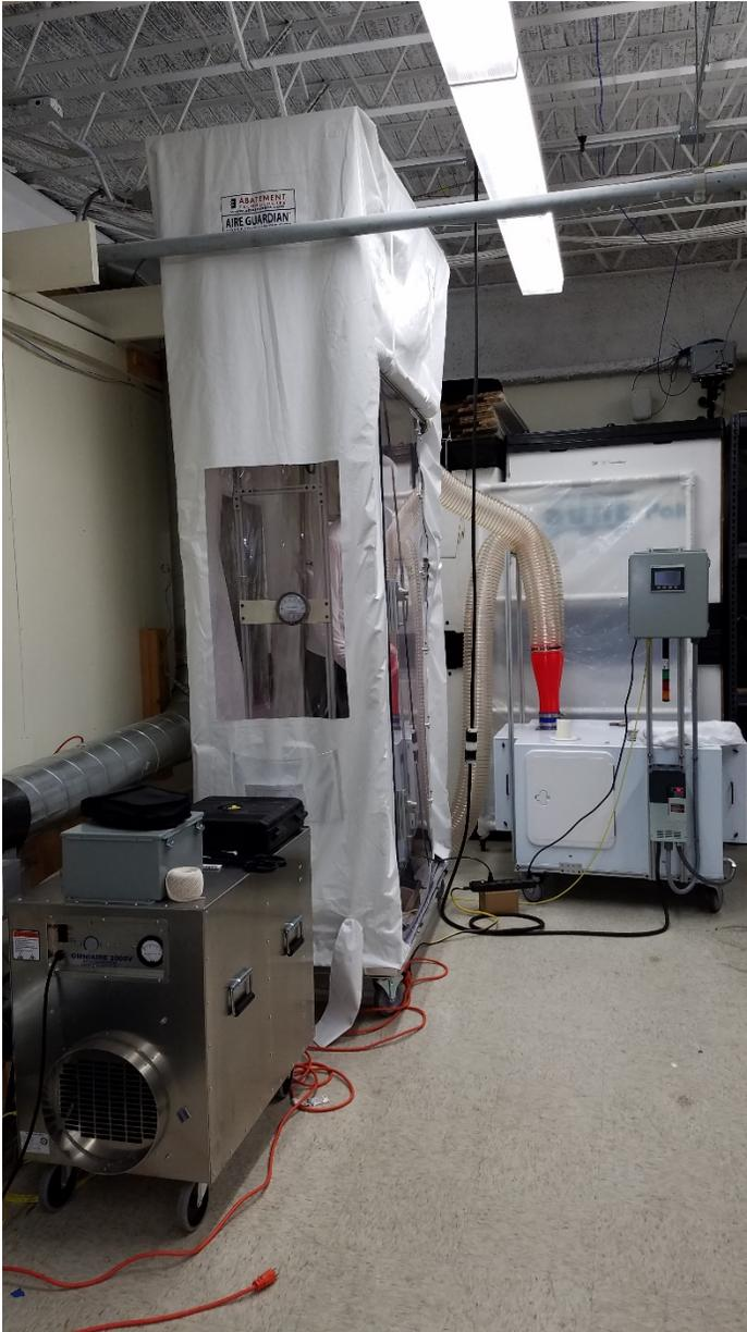
Figure 1. The DryCon system consists of three major components, a HEPA-filtered exhaust blower, a personnel chamber and a positive-pressure blower, from left to right, all mounted on wheels. (Photo credit: NIOSH)
