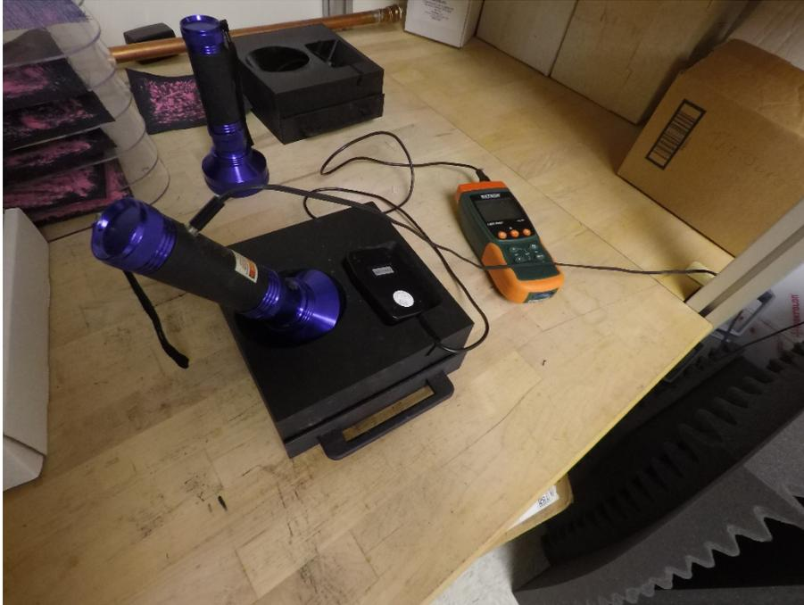
Figure 10. Support used for measuring fluorescence of a fabric swatch, with the swatch drawer closed and the blacklight flashlight and light meter in place. (Photo credit: NIOSH)
