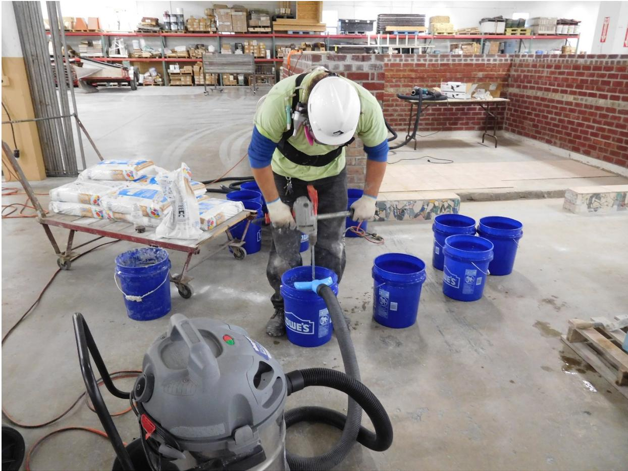
**Figure 5 - Air sampling during thinset mortar mixing (NIOSH photo)**
