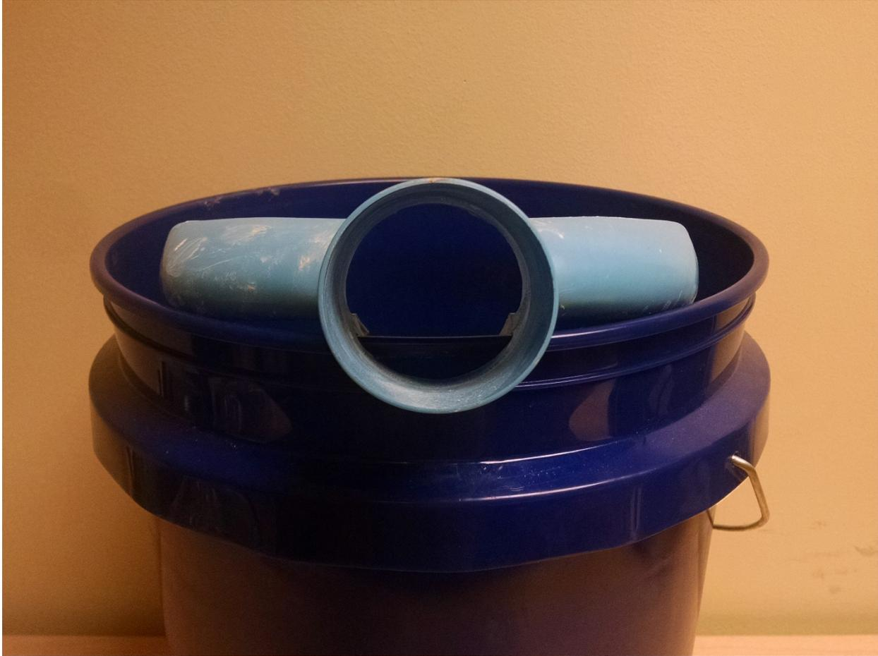
Figure 6 - Rim of the bucket partially occludes hood (NIOSH photo)
