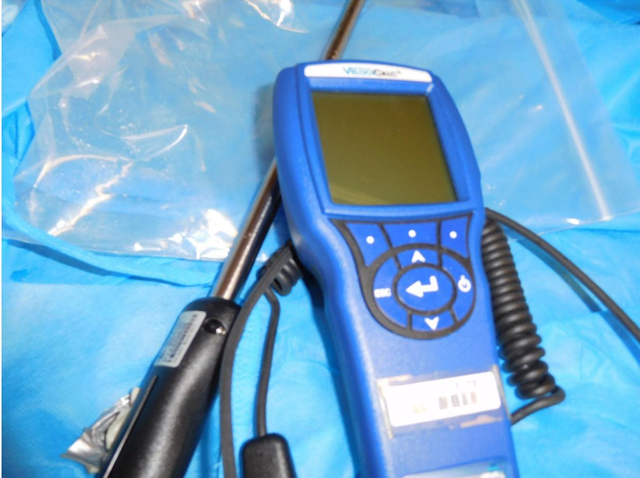
Figure 6. TSI® VelociCalc™ Plus Model 9555-P thermal anemometer (Photo Credit: NIOSH)
