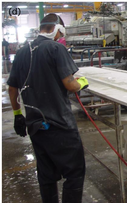
Figure 1 – (a) A worker using a handheld pneumatic wet grinder with a diamond grinding cup wheel in the final grinding process; (b) A worker using a handheld pneumatic wet polisher in the polishing process; (c) A worker using a wet miter saw in the lamination process; (d) A worker using compressed air to dry the surface of the stone in the lamination process.
