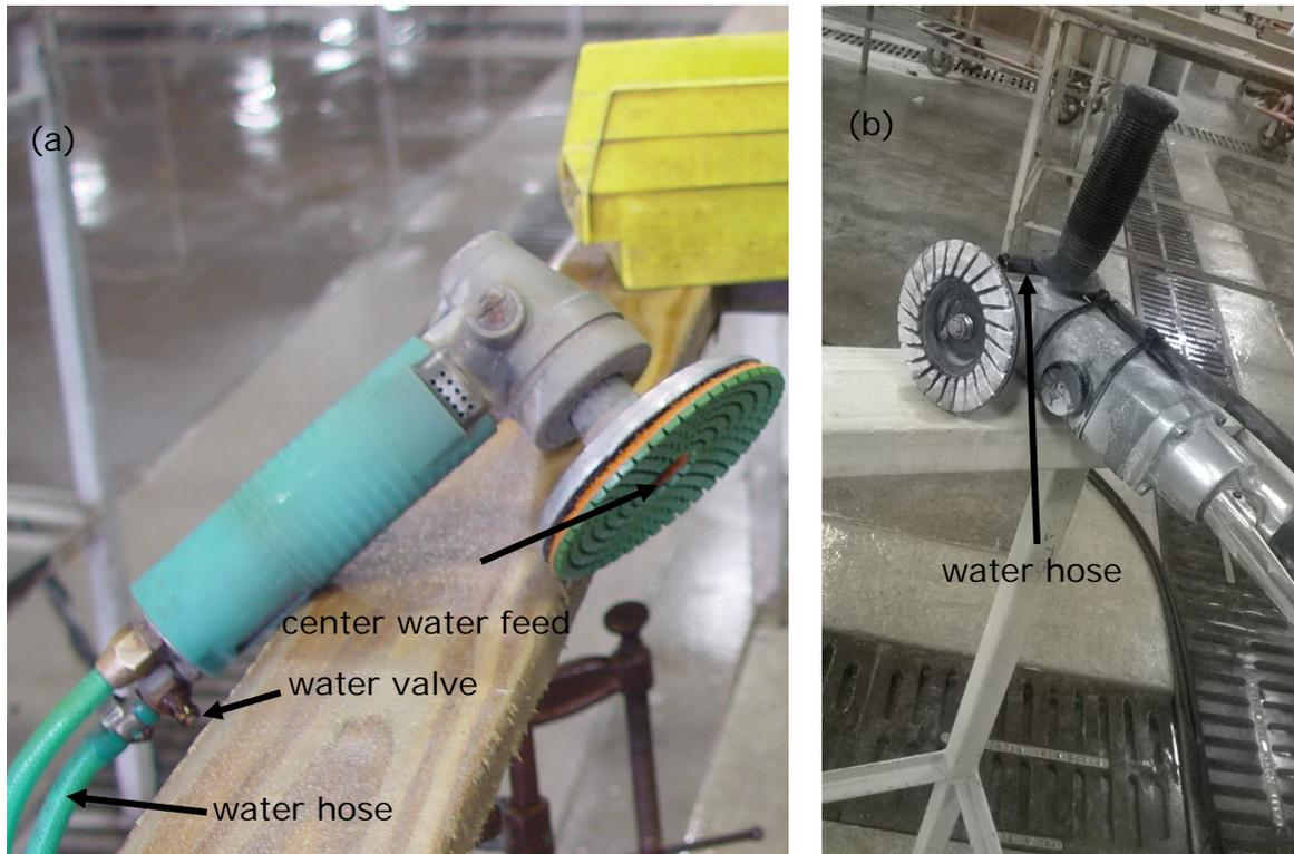
**Figure 2 – (a) A handheld pneumatic wet polisher used in the polishing process; (b) A handheld pneumatic wet grinder with a diamond grinding cup wheel in the final grinding process.**
