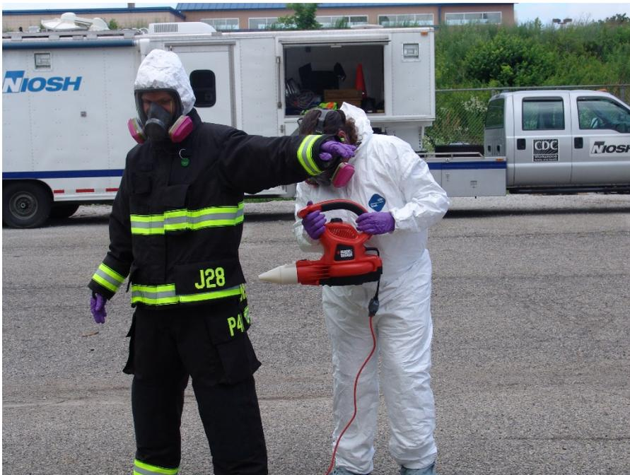
Figure 20. Decontamination trial using leaf blower with short nozzle at the Illinois Fire Service Institute.
