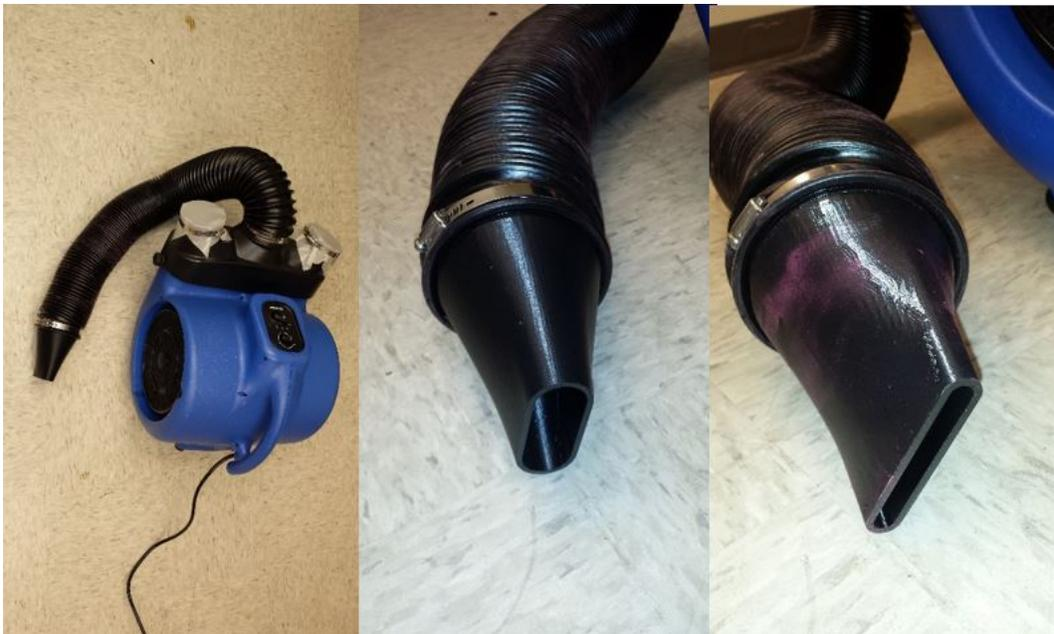
Figure 14. The XPower cage dryer was tested with a wide-slot nozzle and with a narrow-slot nozzle.
