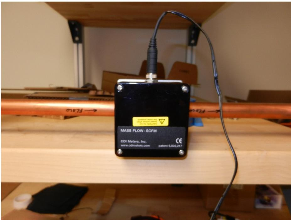
Figure 6. CDI mass flowmeter used to measure the flow rate of compressed air.
