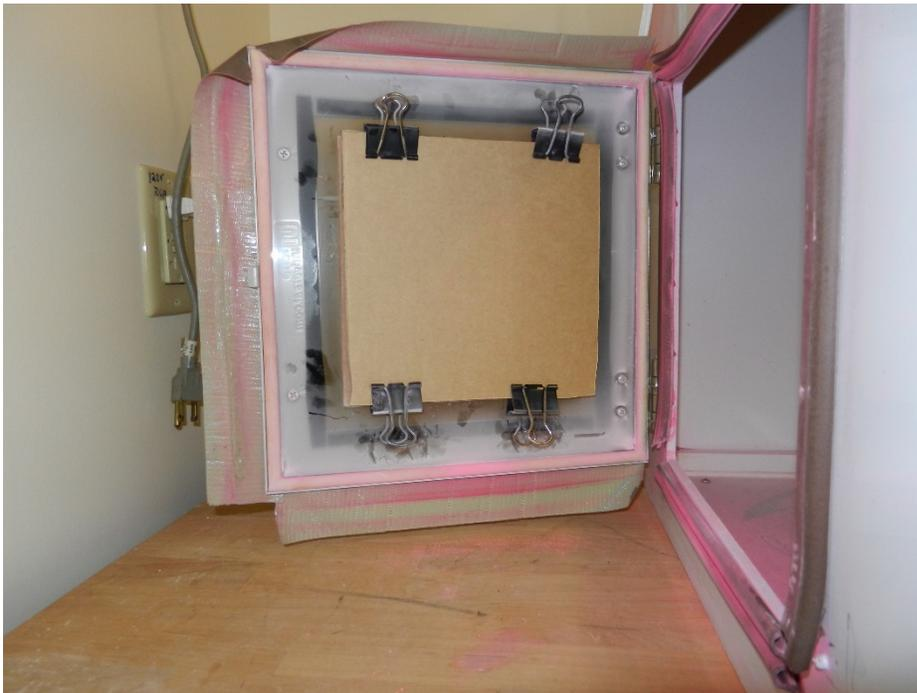
Figure 4. Corrugated cardboard square used for mounting fabric squares for testing.
