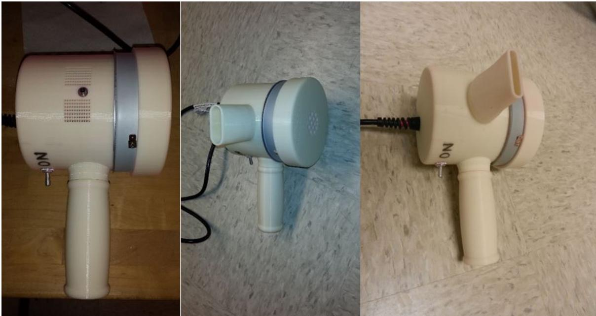
Figure 12. Three different housings tested with high-speed hand dryer blower: outlet holes, wide-slot nozzle and narrow-slot nozzle.
