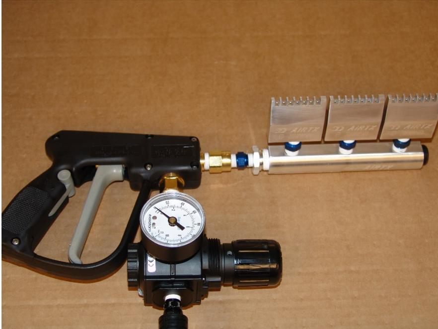
Figure 9. Norgren pressure regulator and Spraying Systems spray gun attached to a manifold with 3 Air TX spray nozzles (configuration 1).
