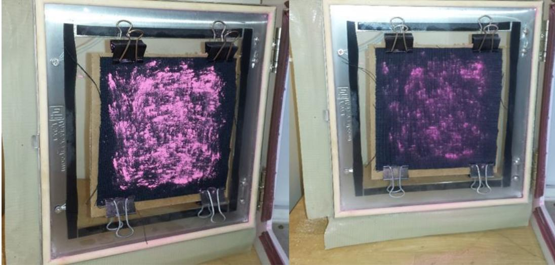
Figure 15. An example of the appearance of the test swatch before and after one of the most successful decontamination trials, using the leaf blower without hose.
