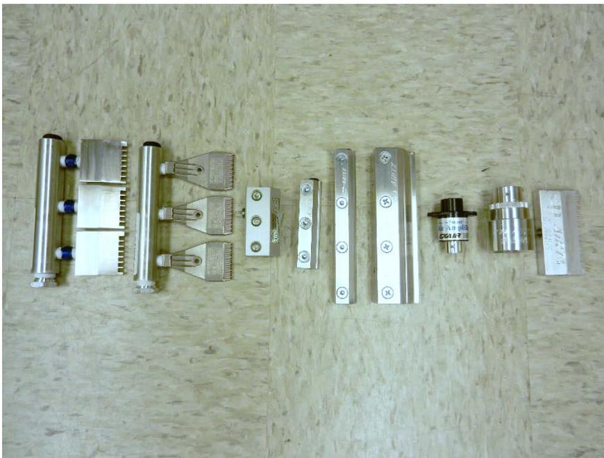
Figure 10. From left to right, air spray configurations 1 - 9, tested with an SCBA cylinder for dry decontamination.
