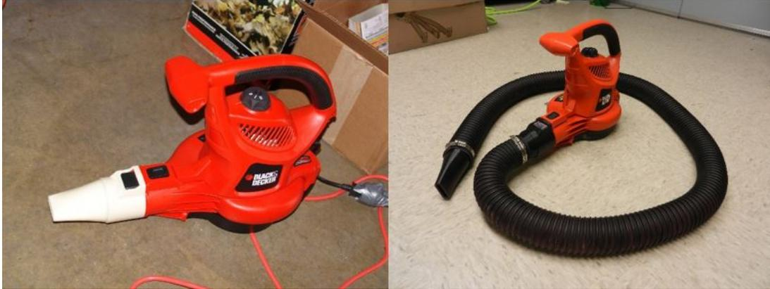
Figure 11. Modified leaf blower used for dry decontamination, with and without hose.
