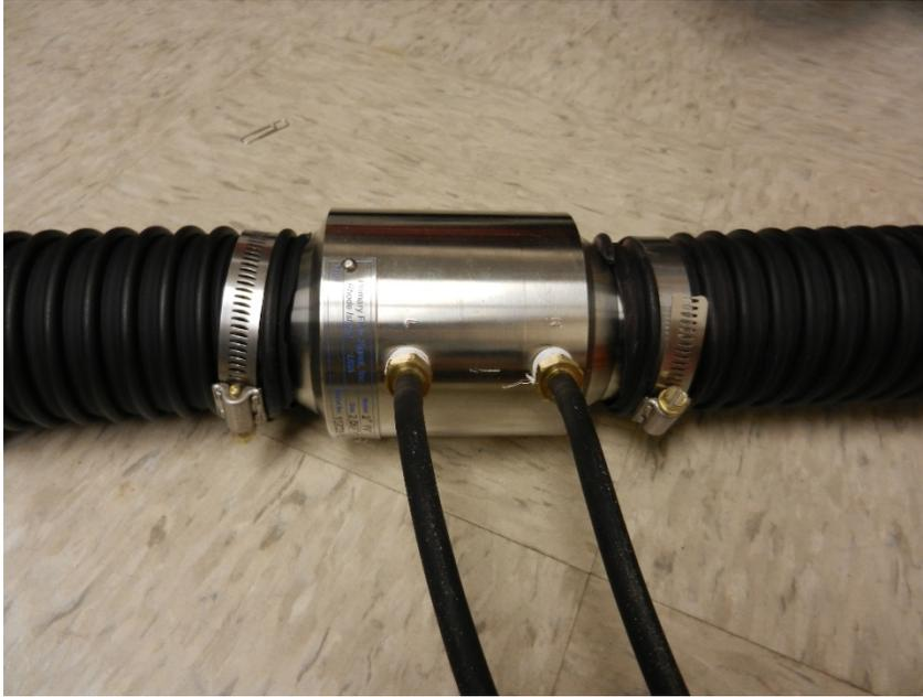
Figure 7. Primary Flow Signal flowmeter, used to measure the flow rate of low-pressure air.
