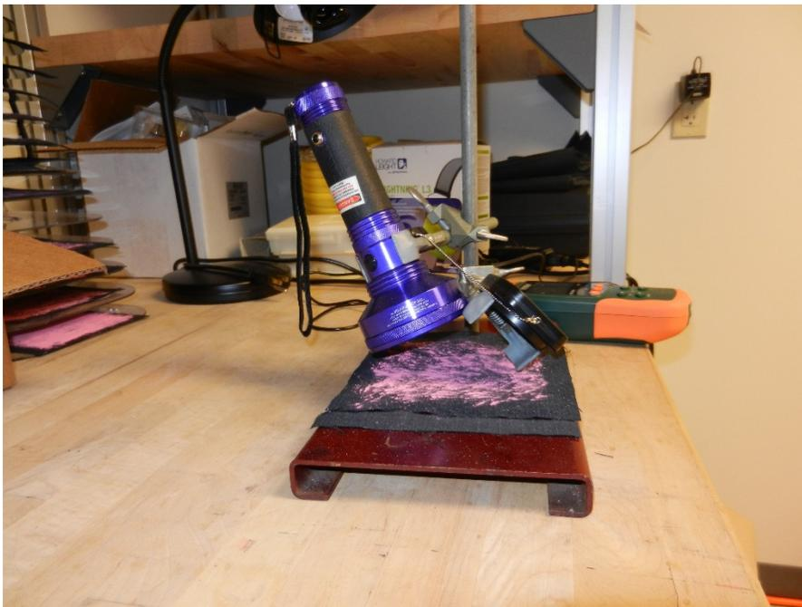
Figure 2. Fabric strips attached to the base of the ring stand allowed fabric squares to be positioned in the same location for each reading.
