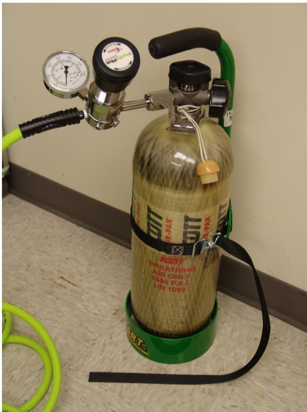
Figure 8. Concoa regulator attached to a Scott breathing air cylinder.
