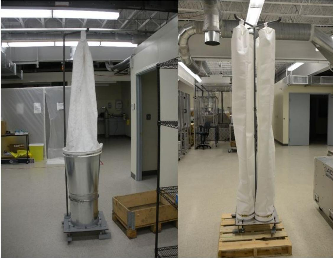
Figure 10. Generation 3 of the mini-baghouse retrofit assembly (right) displays better performance than generation 2 (left). Photos courtesy of Mike Gressel and Jerry Kratzer (left) and Dylan Neu (right).
