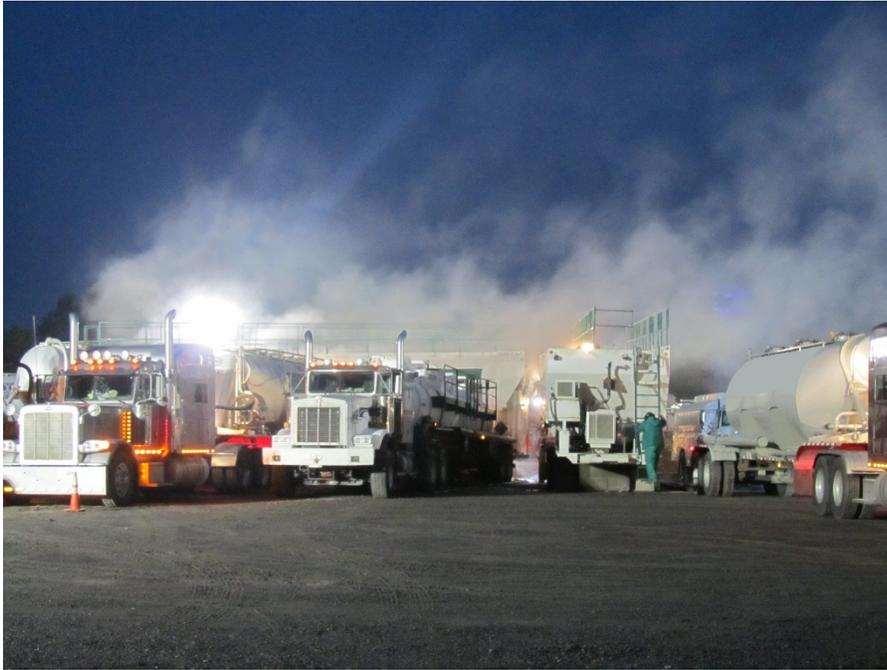
Figure 1. Clouds of dust become visible as sand trucks are unloaded at a hydraulic fracturing site. Photo courtesy of Michael Breitenstein, NIOSH.
