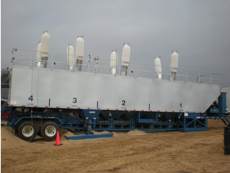
Figure 3. NIOSH mini-baghouse generation 2 assemblies installed on 8 thief hatches atop a sand mover during a 2013 test. Photo courtesy of Mike Gressel and Jerry Kratzer, NIOSH.
