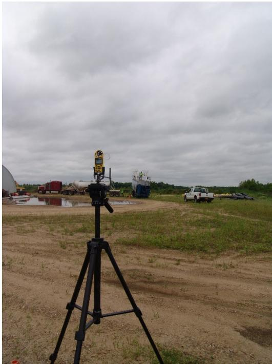
Figure 9. Wind direction and velocity, temperature, and relative humidity were measured with a Kestrel weather meter. Photo courtesy of Barbara Alexander, NIOSH.
