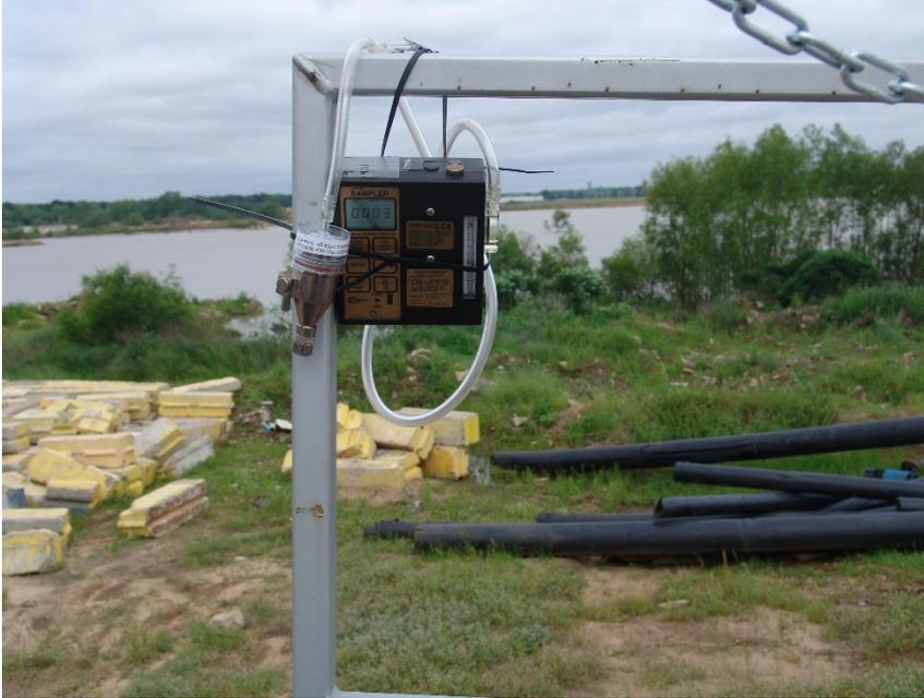
Figure 6. Sampling train installed on upper corner of sand mover. Photo courtesy of Barbara Alexander, NIOSH.
