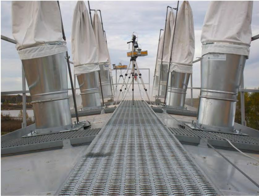
**Figure 9. Mini-baghouse assemblies, including baseplate and sealing surface, ductwork and a 19-inch diameter filter bag. Photo courtesy of Mike Gressel and Jerry Kratzer, NIOSH.**
