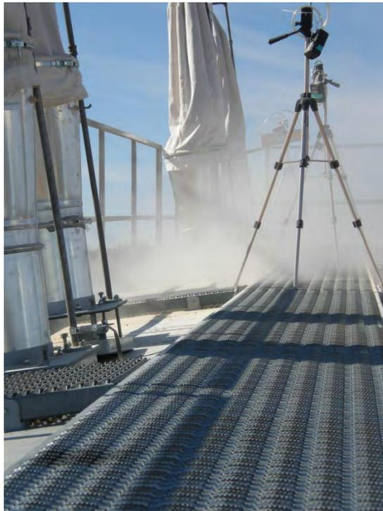
**Figure 6. Sampling train located in the middle of the top of the sand mover during an uncontrolled trial run. Photo courtesy of Mike Gressel and Jerry Kratzer, NIOSH.**
