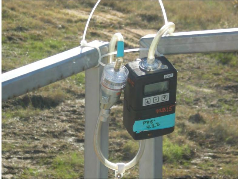
**Figure 5. Sampling train installed on upper corner of sand mover. Photo courtesy of Mike Gressel and Jerry Kratzer, NIOSH.**
