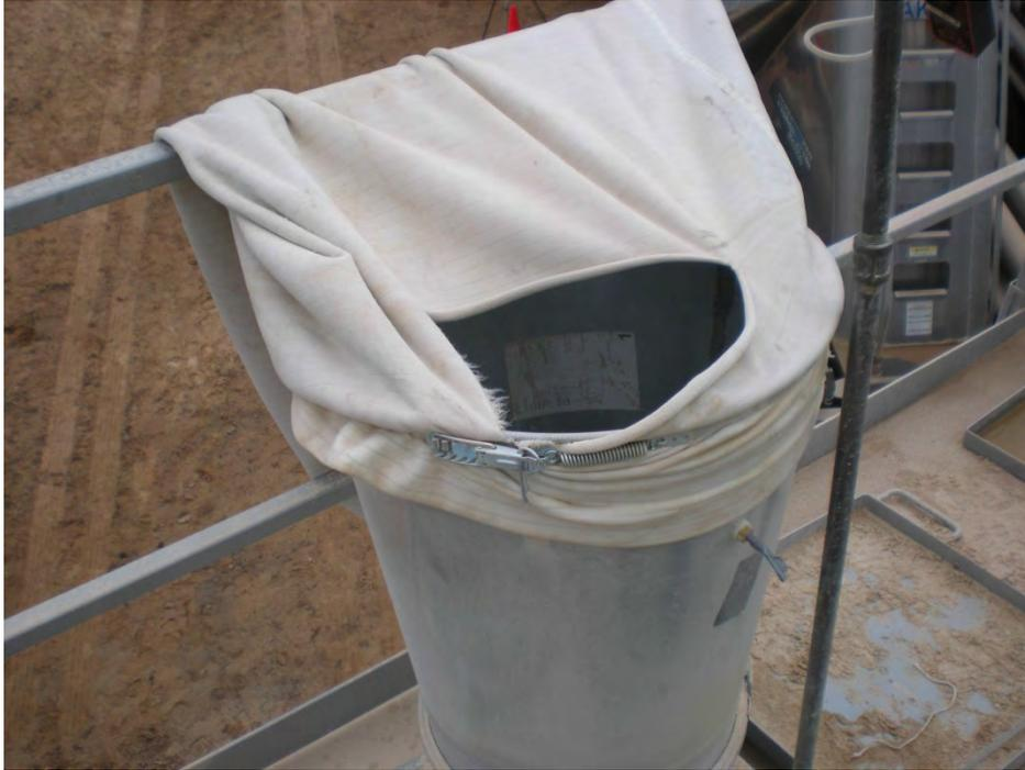
**Figure 21. Failure of filter bag during test of mini-baghouse. Photo courtesy of Mike Gressel and Jerry Kratzer, NIOSH.**
