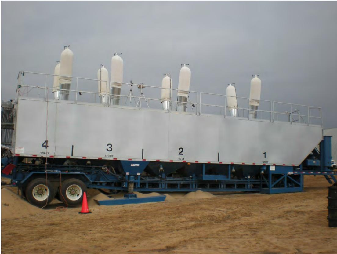
**Figure 3. NIOSH mini-baghouse assemblies installed on 8 thief hatches atop a sand mover. Photo courtesy of Mike Gressel and Jerry Kratzer, NIOSH.**
