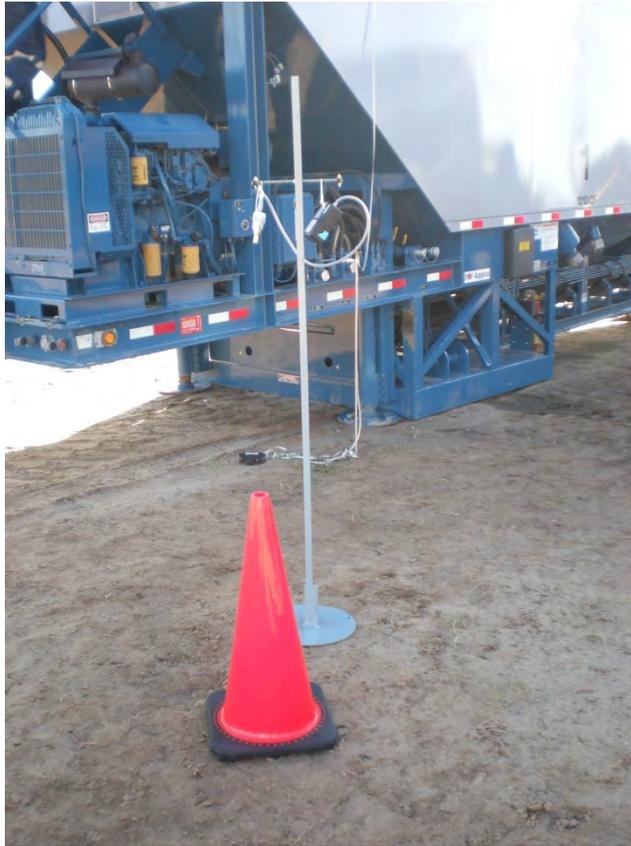
**Figure 7. Sampling train located at breathing zone height on stand next to the sand mover. Photo courtesy of Mike Gressel and Jerry Kratzer, NIOSH.**
