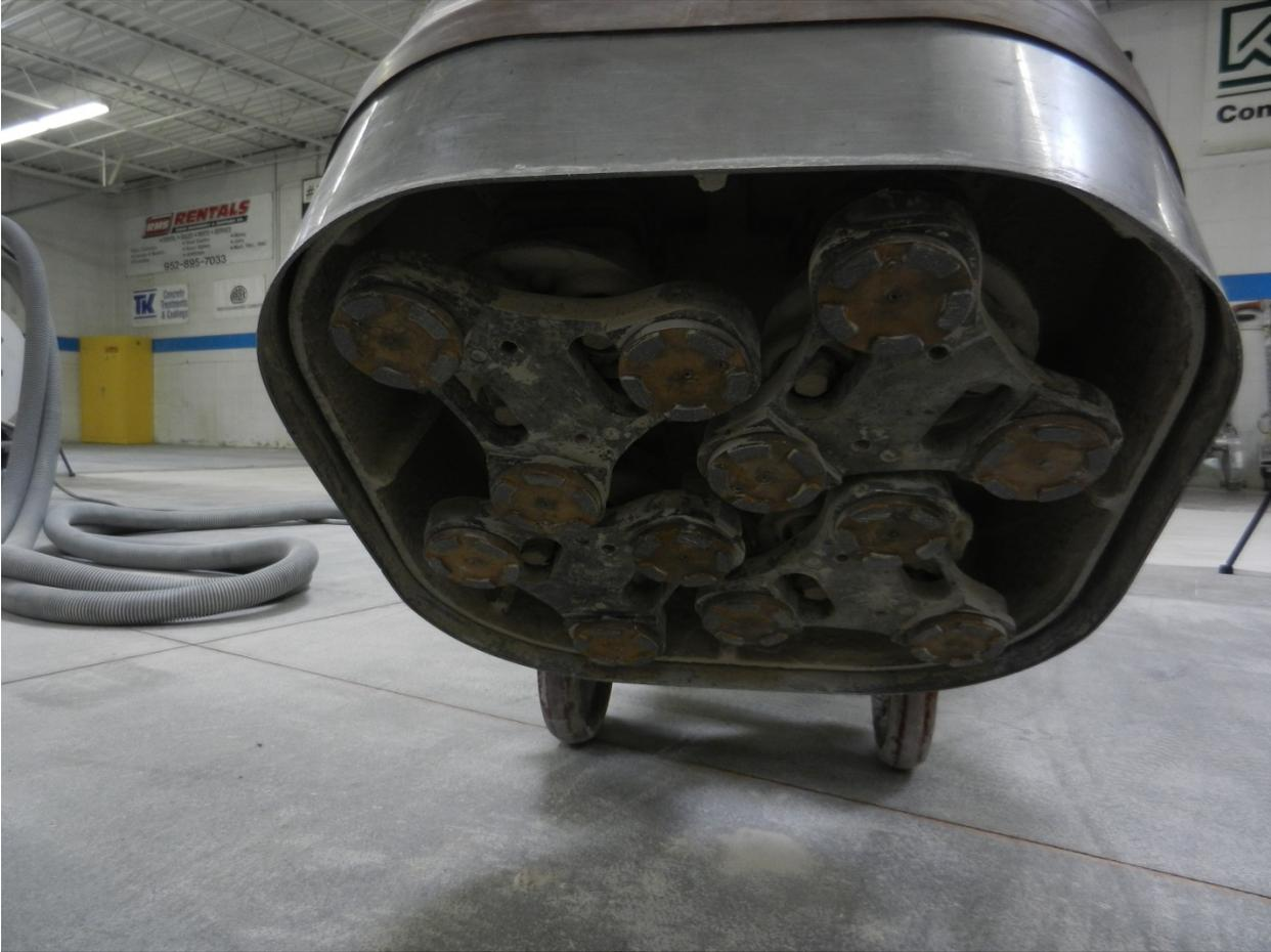
Figure 5: Shroud and polishing disks installed on the Concrete Polisher
