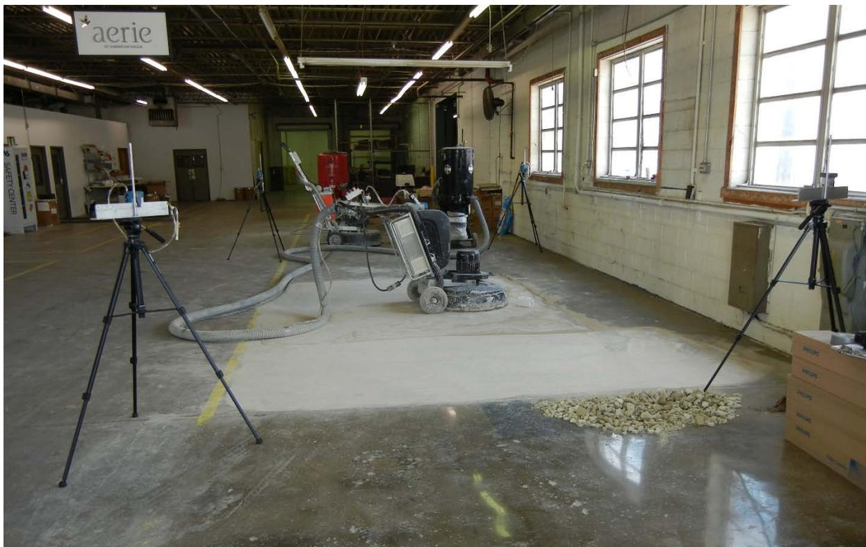
**Figure 3: Polishing area and area sample array**
