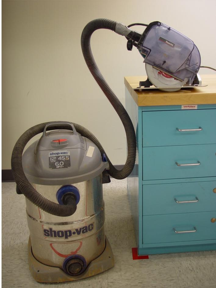
**Figure 3 –The dust-collecting circular saw and its connection to the shop vacuum used in this survey. Photo courtesy of NIOSH.**
