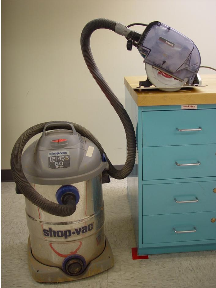
**Figure 4 –The dust-collecting circular saw and its connection to the shop vacuum used in this survey. Photo courtesy of NIOSH.**
