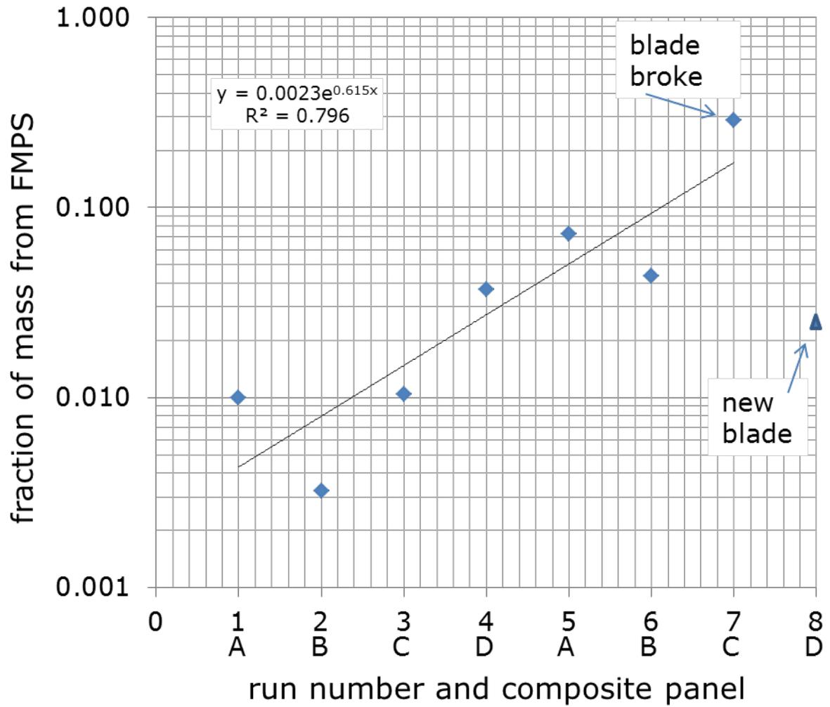
Figure 12. Fraction of mass from the FMPS appears to increase with run number for panel cutting with the band saw.
