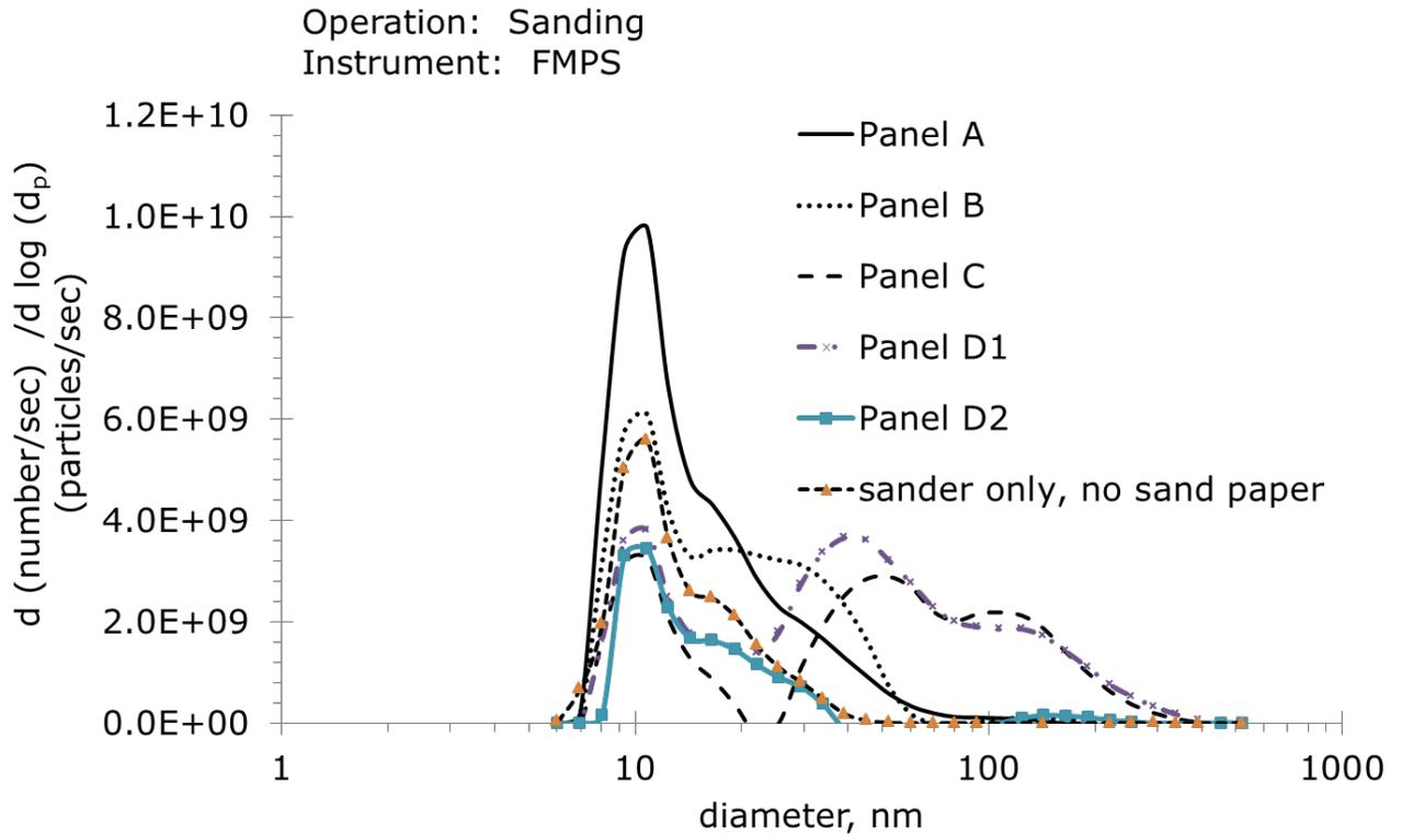
Figure 14. Size-dependent particle number emission rates as a function of particle diameter ( $d_p$ ) measured with FMPS.
