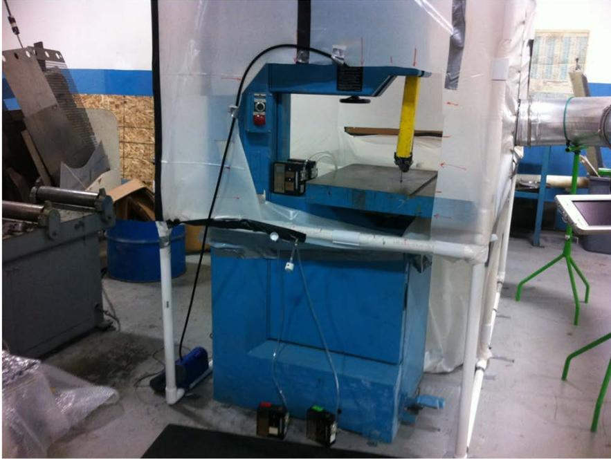
Figure 3. Front view of enclosure around band saw.
