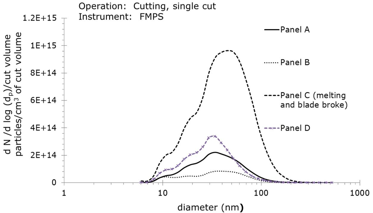
Figure 11. Particle emission rate as a function of particle diameter ( $d_p$ ) measured with the FMPS during second cutting session. When panel C was cut, the saw blade broke and the composite panel partially melted.
