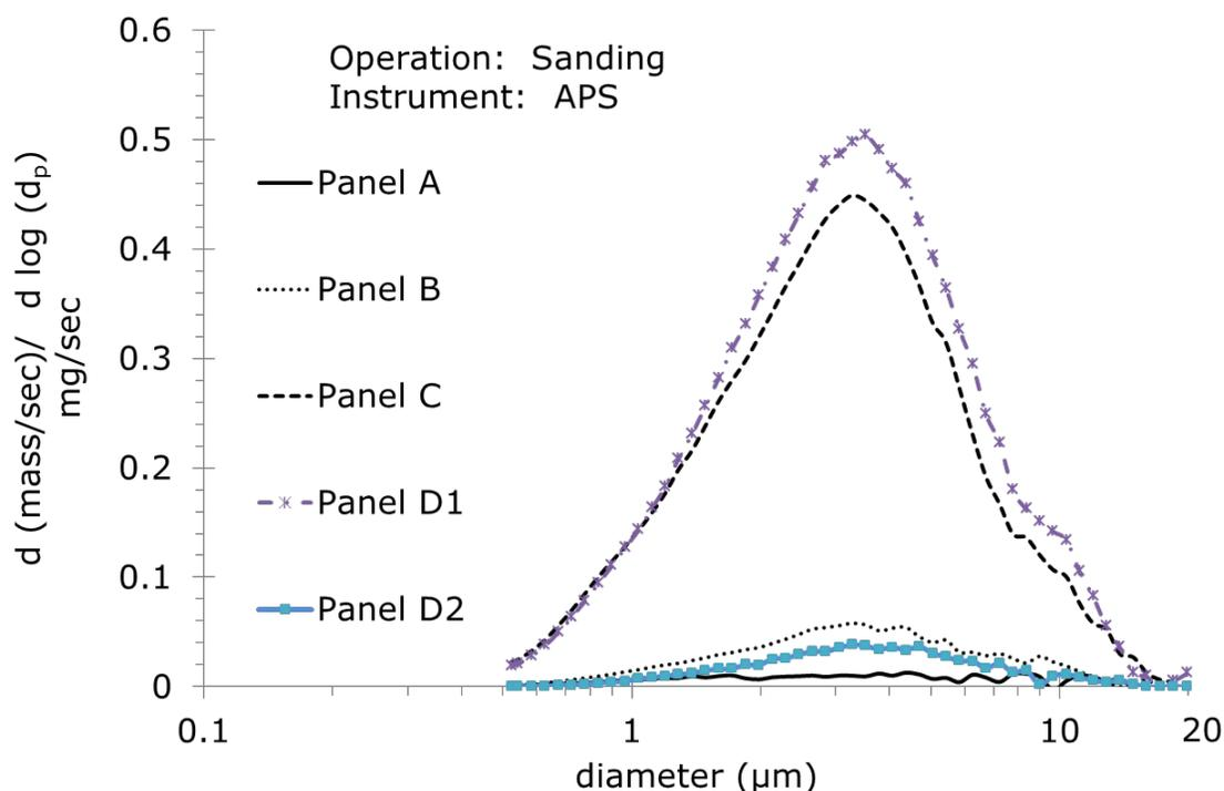
Figure 15. Size-dependent mass emission rates as a function of particle diameter ( $d_p$ ) measured with the APS during sanding.
