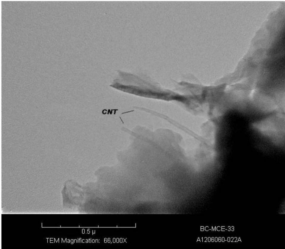
Figure 16. Fiber protruding from debris collected on filter just downstream of the band saw's table during sanding on panel D1.
