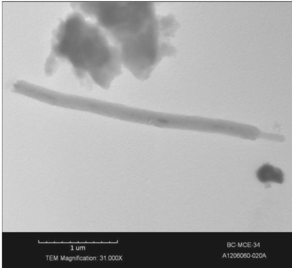
Figure 17. Individual fiber from duct sample collected during sanding of panel D1.
