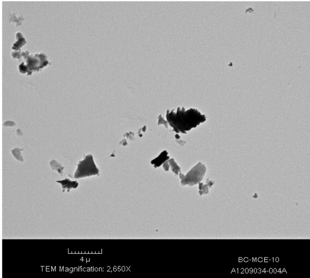
Figure 13. TEM image showing the absence of CNTs or fibers in sample collected in duct during the cutting of composite panel D.
