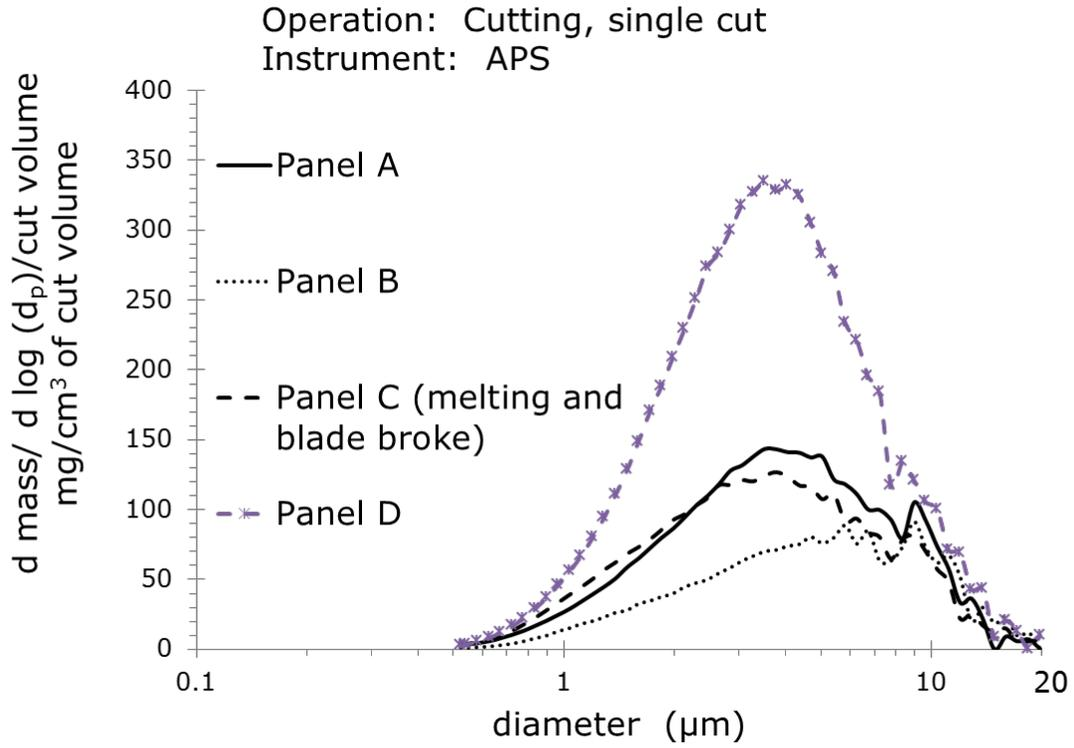
Figure 9. Mass emissions as a function of particle diameter ( $d_p$ ) during the second session with the band saw.
