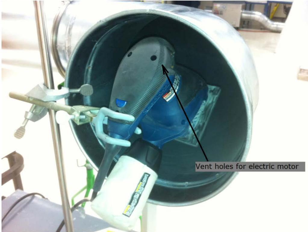
Figure 7. Positioning of the sander at the inlet to the duct.
