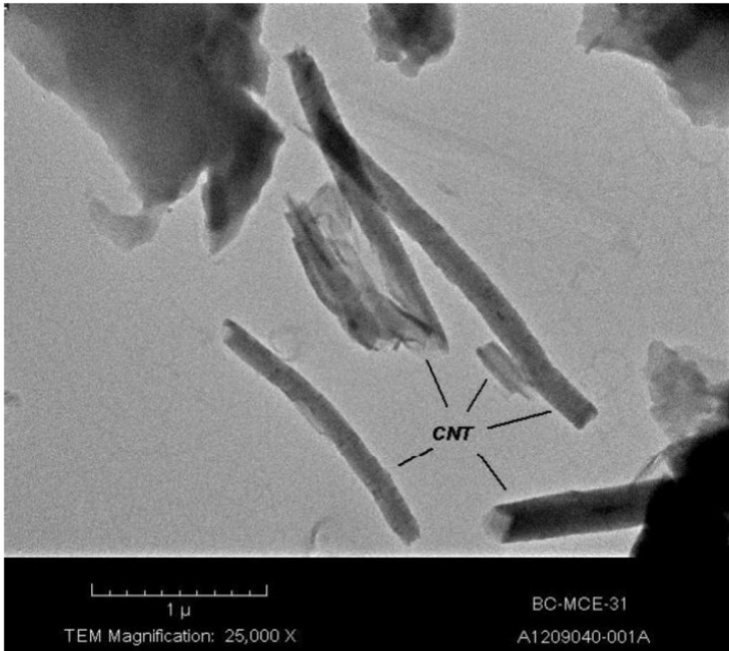
Figure 18. Individual CNTs collected at source for panel D1.
