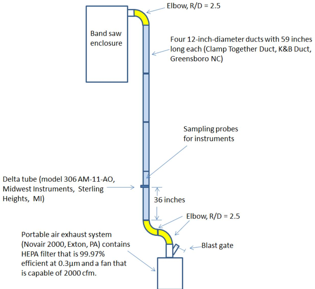
Figure 5. The connecting duct between the enclosure and the portable air exhaust system.
