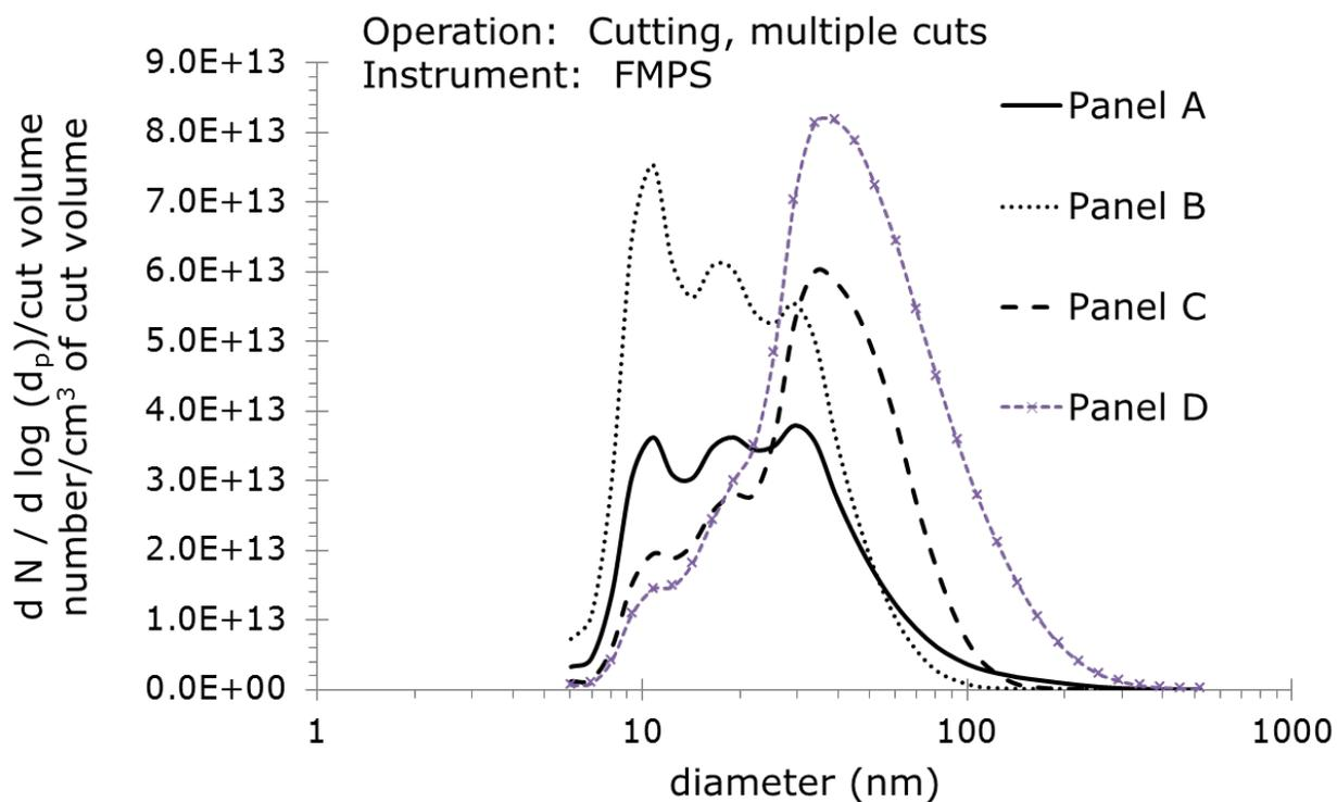
Figure 10. Particle number concentration as a function of particle diameter ( $d_p$ ) measured with the FMPS involving multiple cuts. During the second two cuts there was a shift to a larger particle size.
