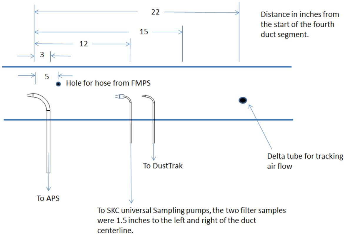
Figure 6. Details of connections between instrumentation and duct.
