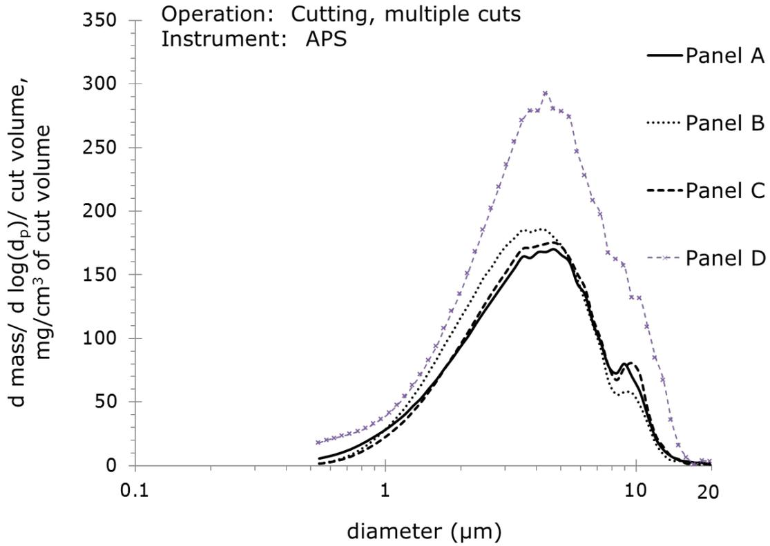
Figure 8. Mass emission rates as a function of particle diameter ( $d_p$ ) from the first session with the band saw.
