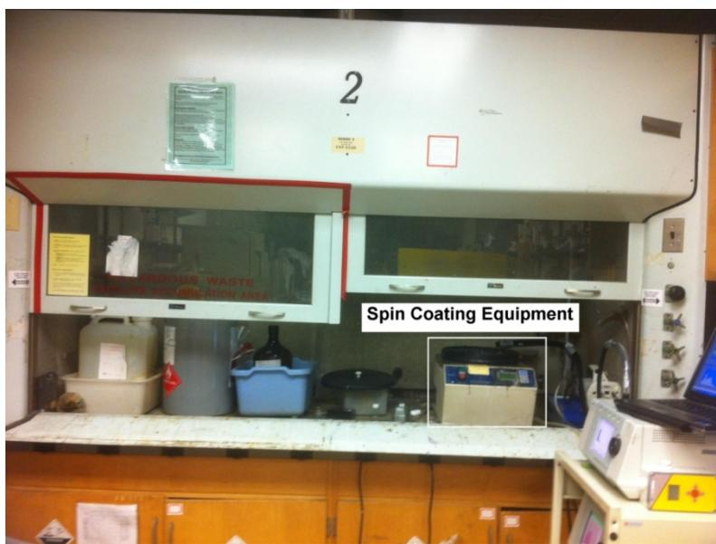
Figure 2. Conventional fume hood used to reduce exposure to nanomaterials during spin coating of CNTs on substrates.
