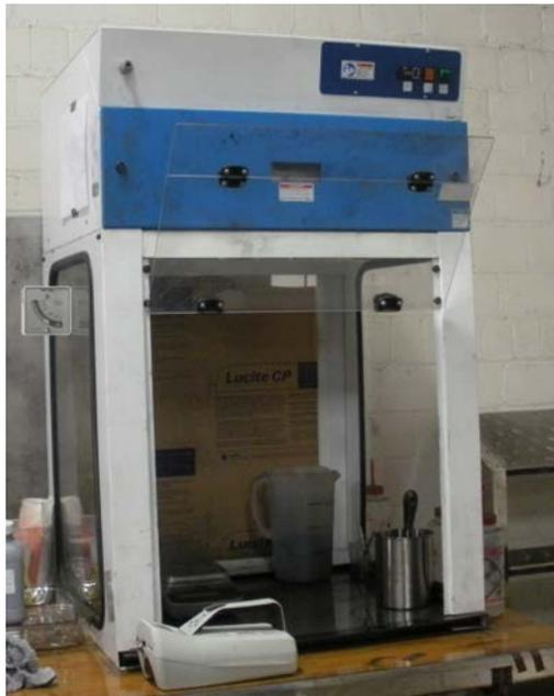
Figure 7. The ventilated enclosure used for product transfer.
