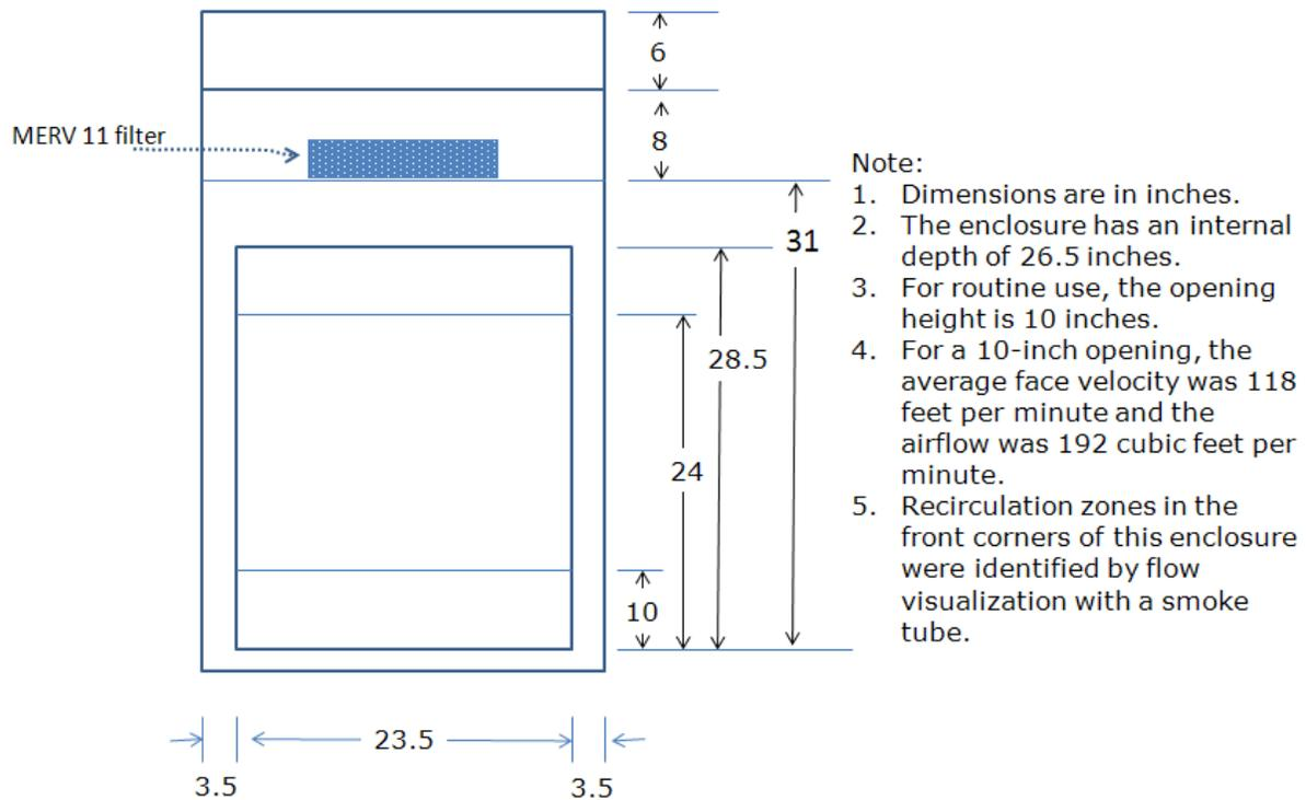
Figure 8. Dimensions of the ventilated enclosure used for product transfer.
