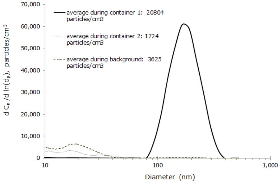
Figure 9. Size-dependent concentrations measured with the FMPS during container removal on 9/26.
