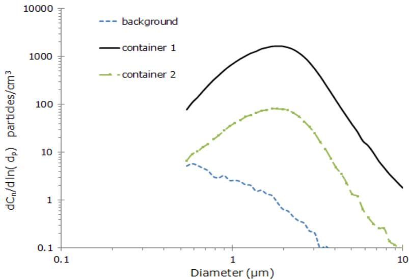
Figure 10. The graphene platelets recovered from the process had aerodynamic diameters larger than 0.5  $\mu\text{m}$ . During disconnection of Containers 1 and 2, the mass concentrations estimated from the APS number concentrations were 9 and 0.4  $\text{mg}/\text{m}^3$  on 9/26.
