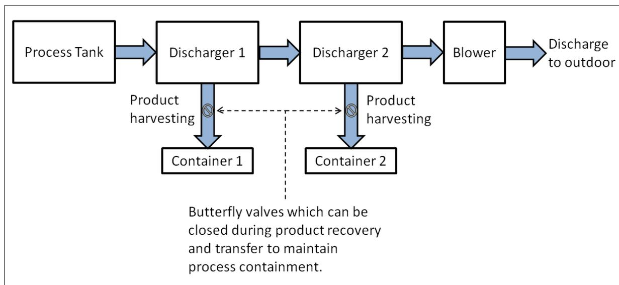
Figure 4. Process Tank 2 used for the refining process. This equipment is smaller than Process Tank 1. It has design features that should minimize dust emissions.
