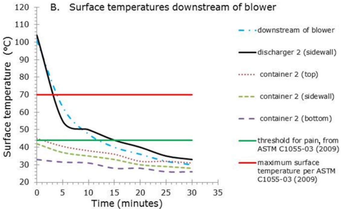
Figure 18. Surface temperature changes on the refining equipment. The temperatures at time = 0 minutes are steady temperatures at the end of the process.
