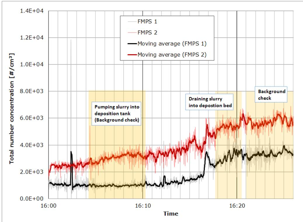
**Figure 11:** Monitoring data for the deposition process with FMPSs on 04/27.
