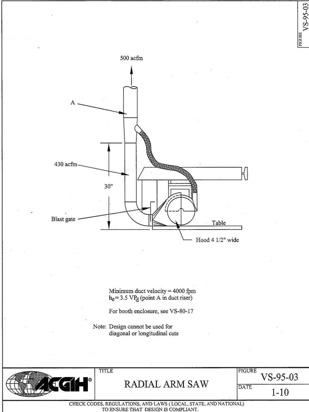
**Figure 19.** LEV designs to control dust emissions from the powered radial saw [ACGIH 2010].
