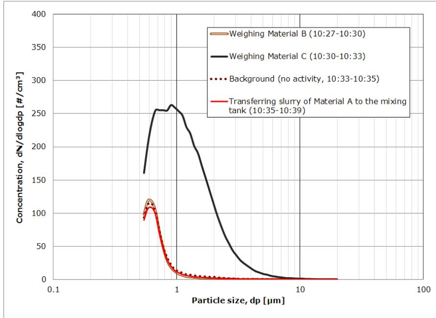
**Figure 10:** Size distribution analysis for the mixing process from 10:27 to 10:39 a.m. on 04/27.
