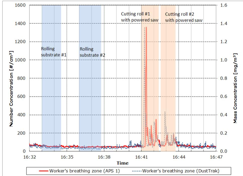
**Figure 12.** Process monitoring by (a) FMPSSs, and (b) APS 1 and DustTrak, for rolling substrates on the downdraft table and cutting rolls by the powered circular saw with the canopy hood off (normal operation) on 04/27.
