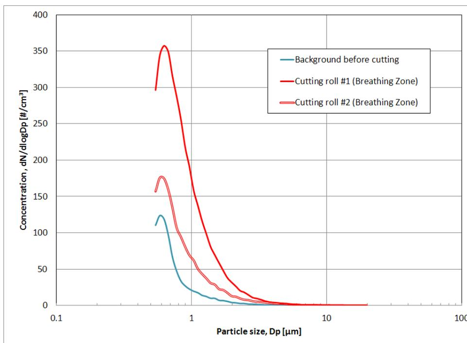
**Figure 13.** Particle size distribution analysis from (a) FMPSs and (b) APS 1 during the cutting of substrate rolls using the powered circular saw.
