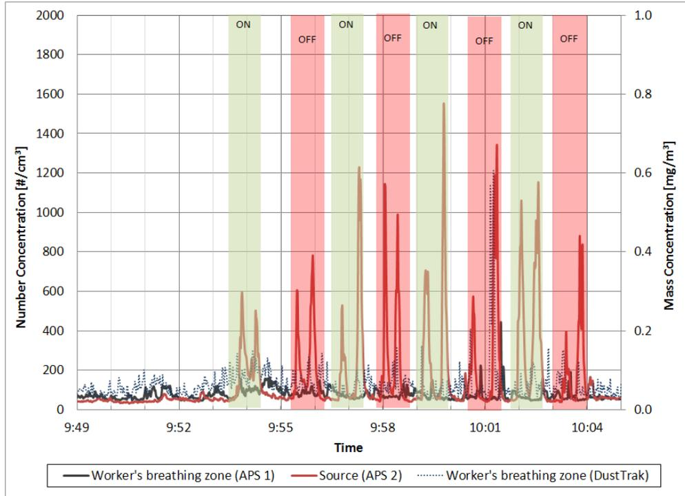
**Figure 14.** Particle concentration monitoring data of (a) FMPSSs, and (b) APSs and DustTrak during the evaluation of the canopy hood used for the powered saw cutting.
