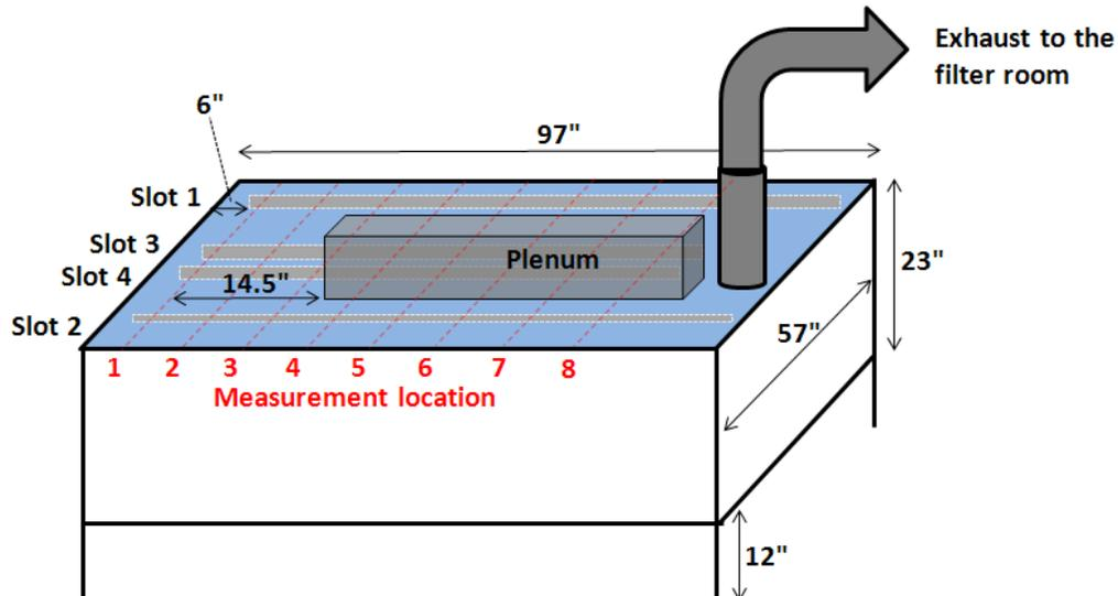
**Figure 5:** Top view of the downdraft table.
