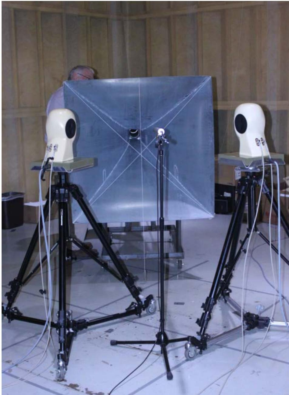
Figure 1: E-A-RCAL and NIOSH acoustical test fixtures located on the left and right of the blast probe facing the catenoidal horn.
