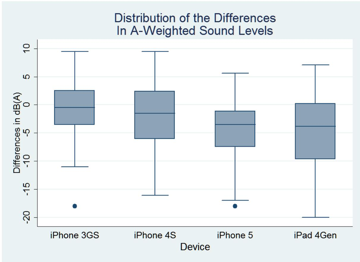
**Figure 5. Box plots of differences in A-weighted sound levels (dBA) between reference microphone and app measurements by device.**
