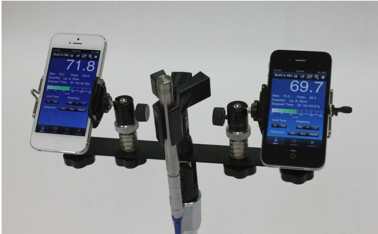
**Figure 2. The SoundMeter app on the iPhone 5 (left) and iPhone 4S (right) compared to 1/2" Larson-Davis 2559 random incidence type 1 microphone (center).**
