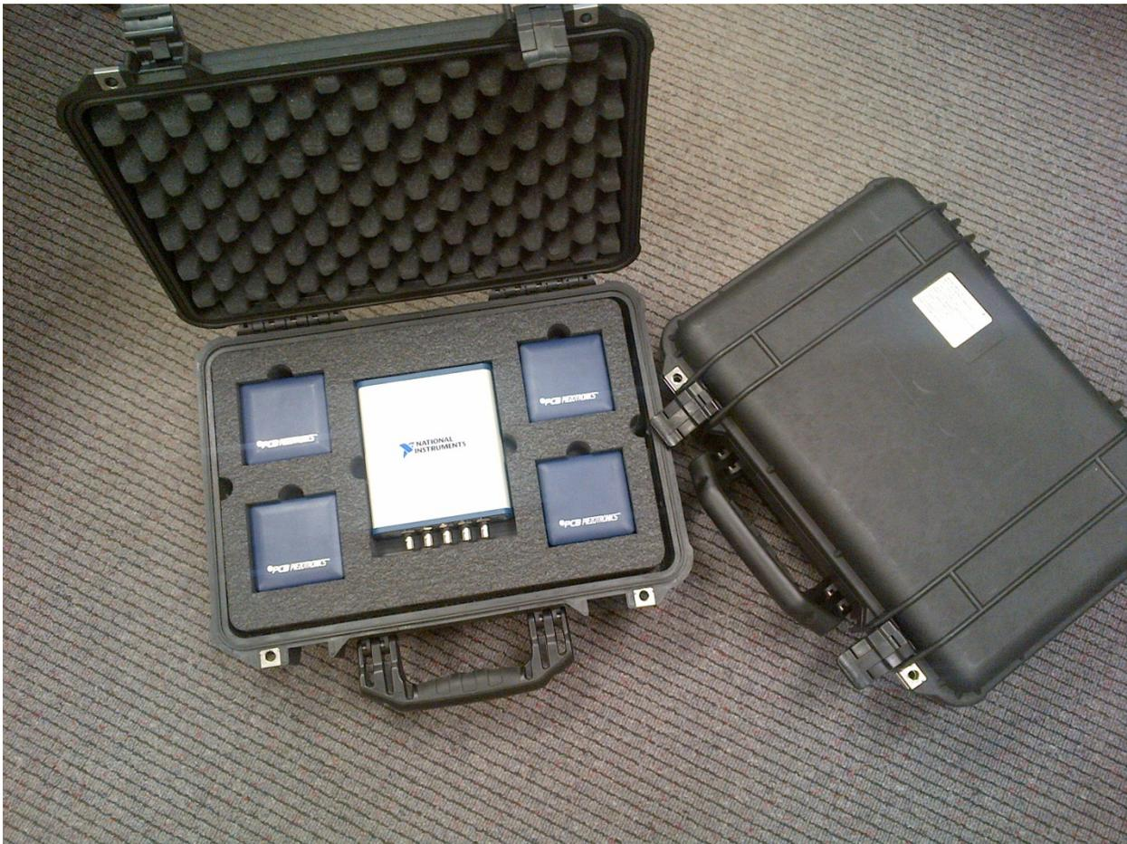
**Figure 1. NIOSH Impulsive Noise Measurement Kit**
