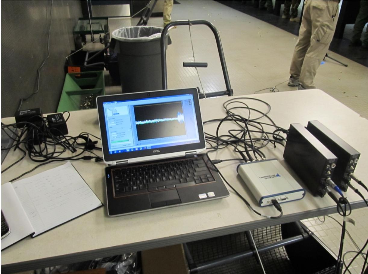
**Figure 2. The NIOSH Impulsive Noise Meter Setup**
