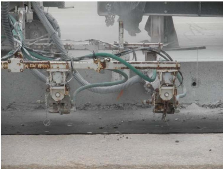
**Figure 6 - The Exhaust Hose Sags in Horizontal Runs Near the Hoods**
