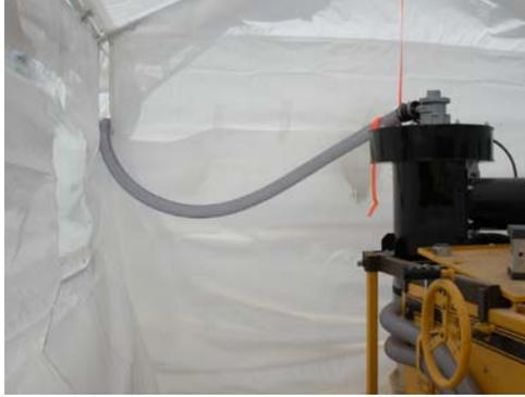
Figure 3 - The exhaust from the pneumatic fan motor was routed outside the tent
