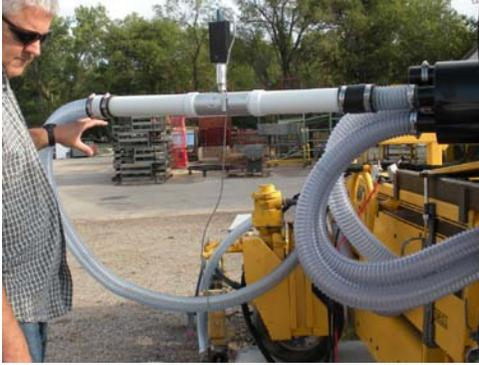
Figure 7 - Exhaust ventilation measured with meter in line
