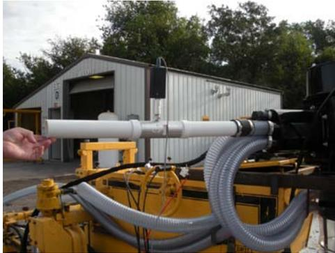
Figure 6 - Exhaust ventilation measured at collector with hose disconnected
