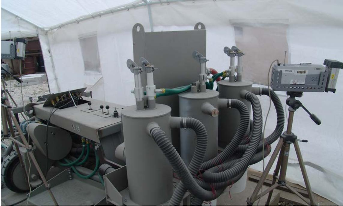
Figure 5: Sampling Instruments were Placed at Three Locations. The operator's platform is at the lower left of the photograph. The dust collectors are in the center of the photograph. The rear sampling position is at the right. The operator stands on the platform while driving the dowel drilling machine. Because the drills stop at a pre-set depth, the operator can start the drills and step away from the dust cloud.
