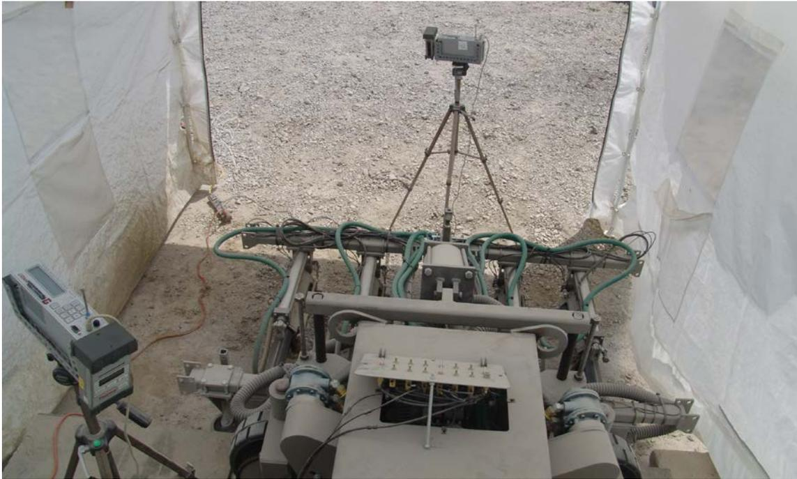
Figure 4: Sampling Instruments were Placed on Tripods at Breathing Zone Height. This photograph shows the front (top) and operator (left) sampling positions.
