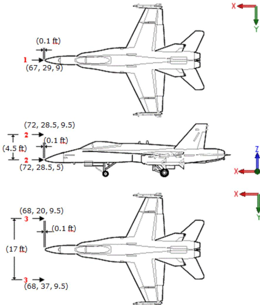
**Figure 3: Source locations (x,y,z) in feet, relative to the origin shown, for the release of SF<sub>6</sub> near the front of the F/A-18C/D Hornet. Source: <http://www.boeing.com/defense-space/military/fa18/fa18cd3v.htm>**
