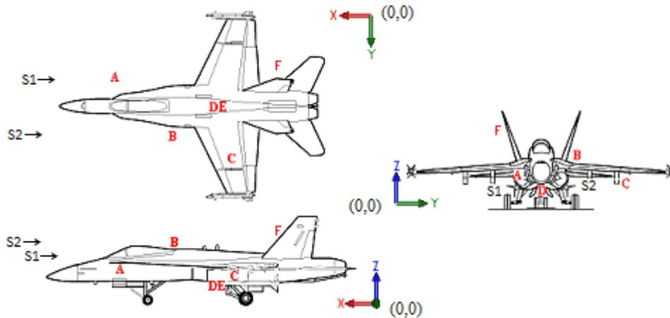
Figure 8. Source and sample locations for the release of SF<sub>6</sub> near the front of the F/A-18C/D Hornet. Source: <http://www.boeing.com/defense-space/military/fa18/fa18cd3v.htm>
