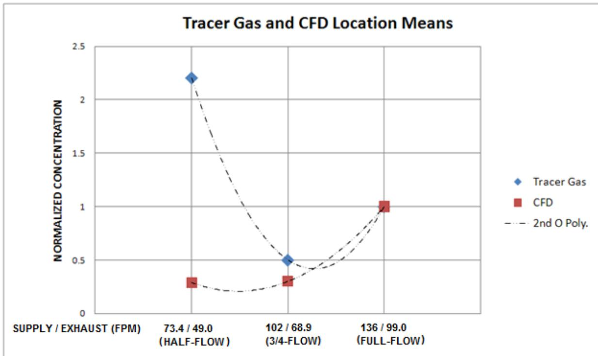
**Figure 9: Five-location-mean concentrations for CFD simulations and tracer gas experiment means, as a function of flow rate.**
