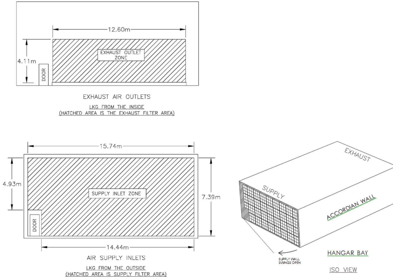
Figure 1. Drawing showing filter area of Bay 6, Building 465, Fleet Readiness Center Southwest, San Diego, CA.
