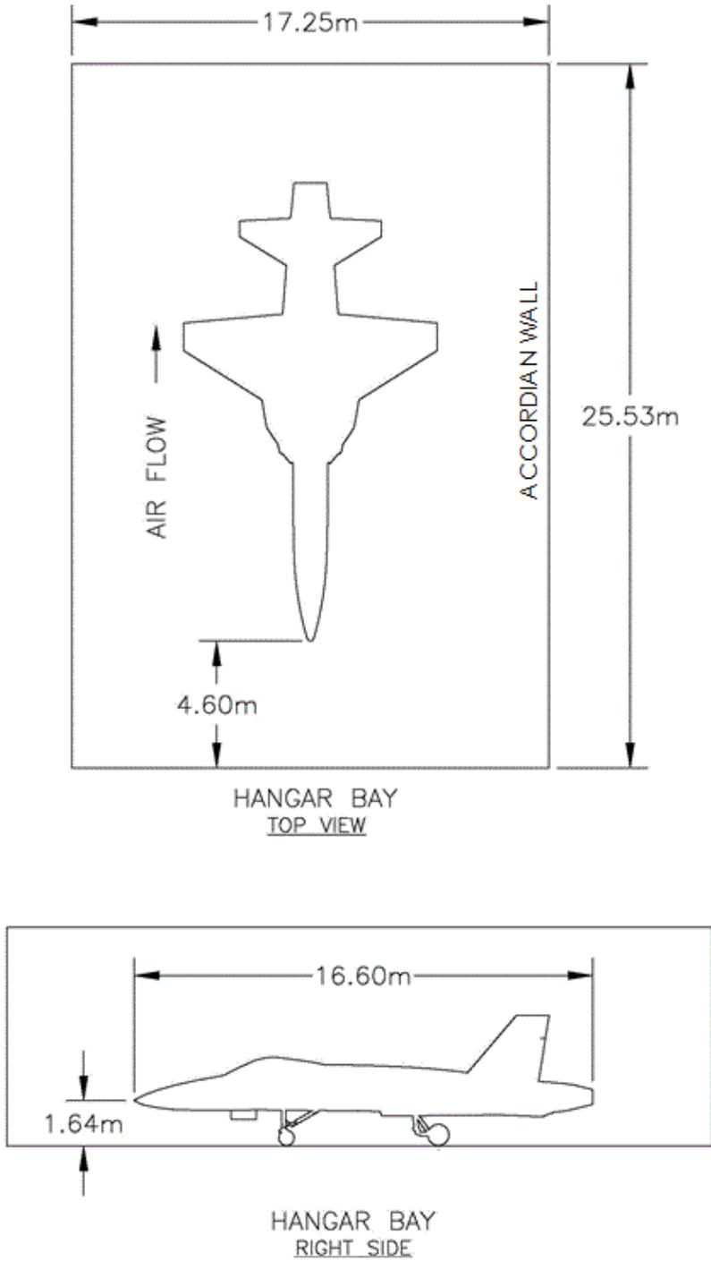
Figure 2. Drawing showing interior of bay and F/A-18C/D Hornet. Bay 6, Building 465, Fleet Readiness Center Southwest, San Diego, CA.
