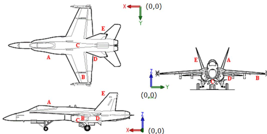
Figure 4: Approximate locations of the five MIRAN<sup>®</sup> Sapphires around the F/A-18C/D Hornet during the first release scenario. Source: <http://www.boeing.com/defense-space/military/fa18/fa18cd3v.htm>
