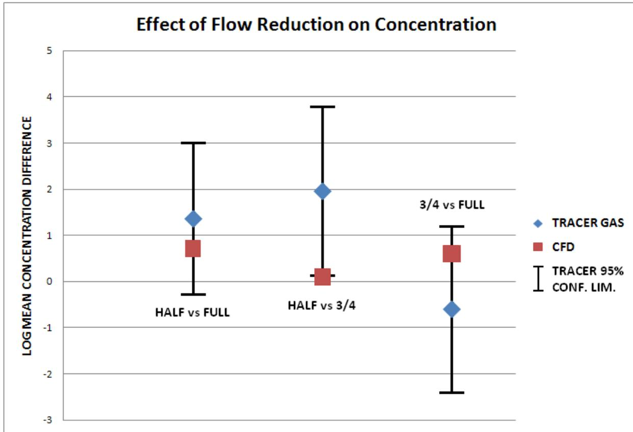
Figure 10: Flow rate comparison by CFD and tracer gas methods.
