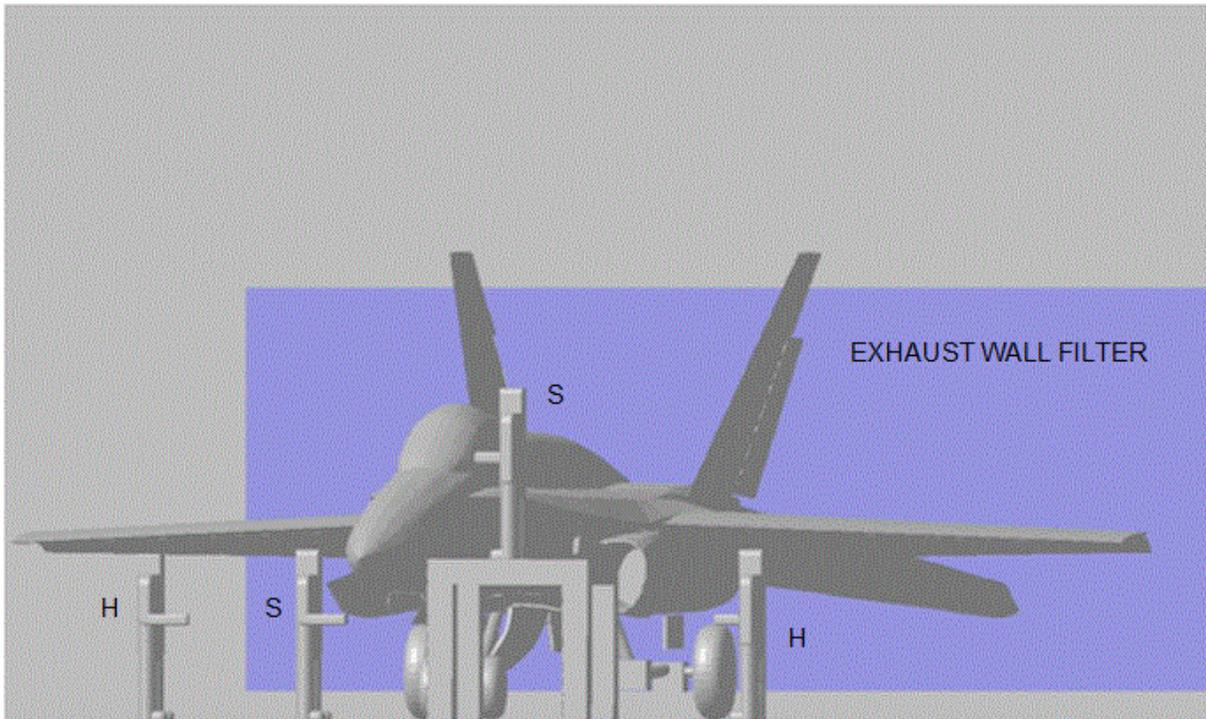
**Figure 7. Geometry of workers, exhaust wall filter, and F/A-18C/D Aircraft. Hosemen (H) are further from the aircraft and further downwind than sprayers. The contaminant source is located at the end of the sprayers' (S) right arms. One sprayer is on a scaffold.**
