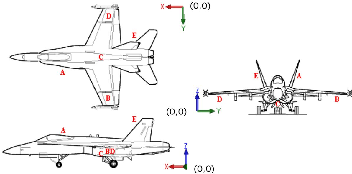
Figure 8: Approximate locations of the five MIRAN<sup>®</sup> Sapphires around the F/A-18C/D Hornet during the second and third release scenarios. Source: <http://www.boeing.com/defense-space/military/fa18/fa18cd3v.htm>
