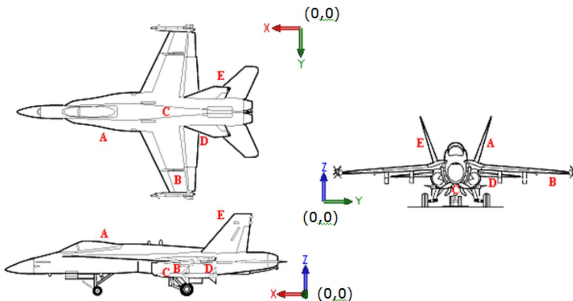
Figure 7: Approximate locations of the five MIRAN<sup>®</sup> Sapphires around the F/A-18C/D Hornet during the first release scenario. Source: <http://www.boeing.com/defense-space/military/fa18/fa18cd3v.htm>
