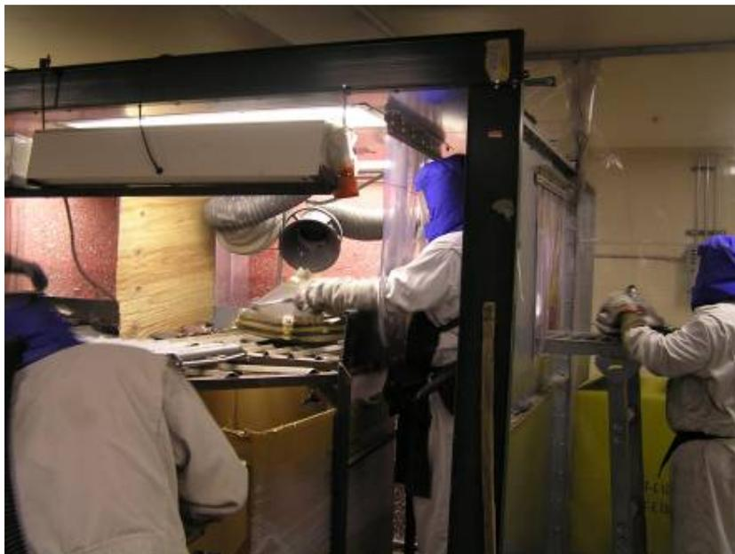
Figure VIII – Filter Change Operation in Glass Breaking Area
