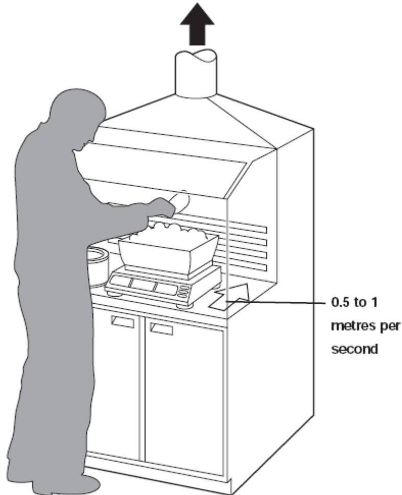
Figure 6. Welding Ventilation Bench Hood.
