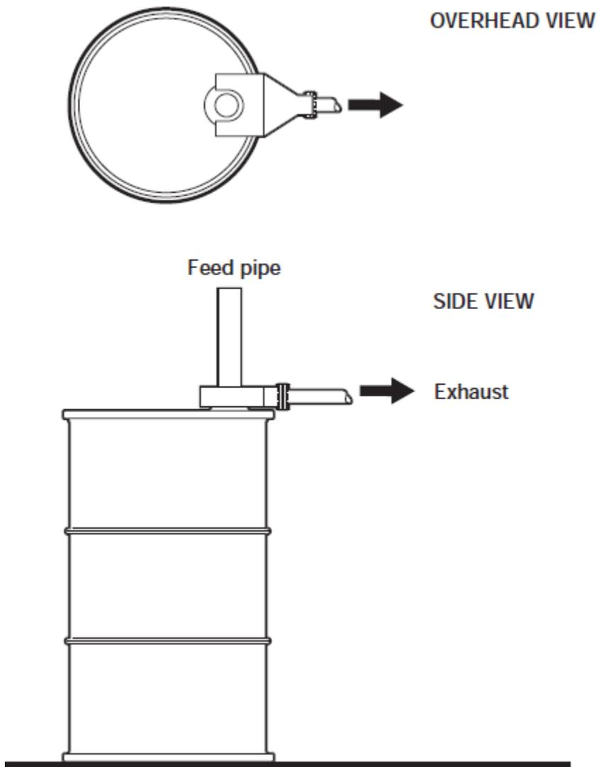
**Figure 4. Ventilation Design Options for Capturing Vapors During Drum Filling/Emptying\***
