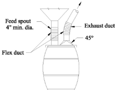
$Q = 50 \text{ cfm} \times \text{drum diam. (ft)}$
