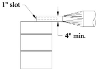
$Q = 100 \text{ cfm/ft}^2$  barrel top (minimum)
