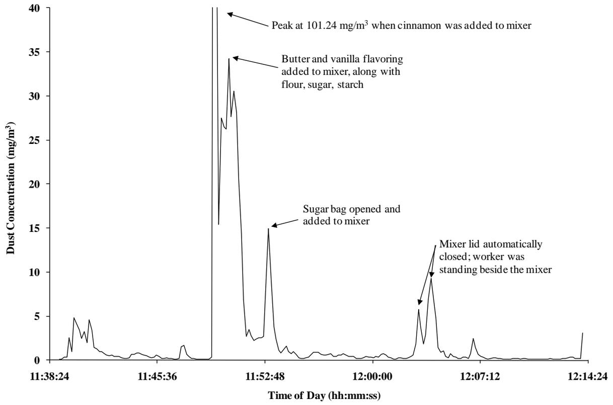
Figure 2. Real-time Data for Cinnamon Smear Dust
