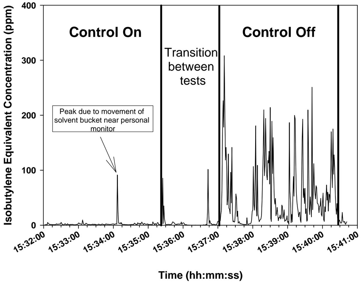
Figure 9. Real-time evaluation of bench top exhaust hoods--control on/off.
