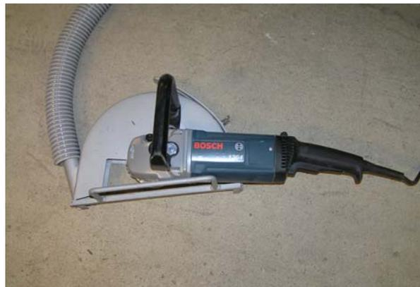
**Figure 2: Bosch Hand-held Electric-powered Saw**
