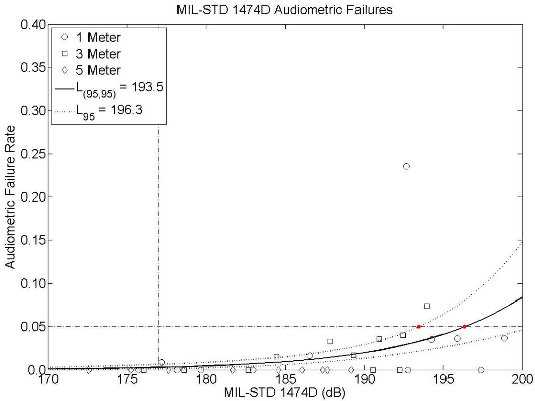
Figure 2: Evaluations of 1, 3 and 5-meter exposures using the MIL-STD-1474D metric using the audiometric and conditional failures. The logistic regression curve and 95% confidence intervals are shown as the solid and dotted lines. The  $L_{(95,95)}$  and  $L_{95}$  points are plotted with a solid dot symbol. The 5% failure criterion and the 177 dB design limit are shown as horizontal and vertical dashed-dotted lines.
