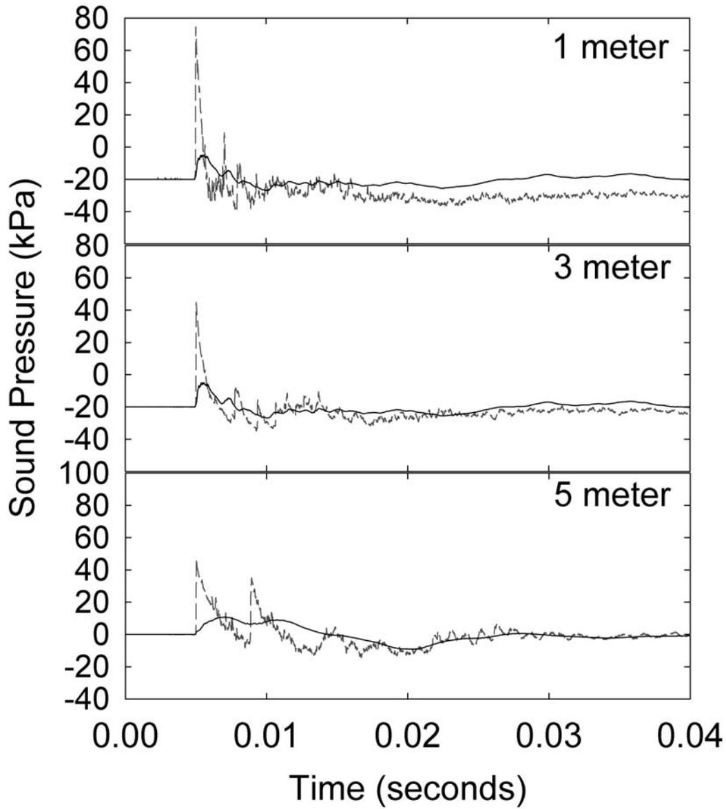
Figure 1: Example waveforms from the 1, 3 and 5-meter exposures for the free-field (dashed line) and protected (solid line) conditions.
