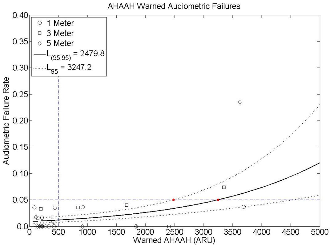
Figure 10: Evaluations of 1, 3 and 5-meter exposures using the warned AHA AH model using the audiometric failures. The logistic regression curve and 95% confidence intervals are shown as the solid and dotted lines. The  $L_{(95,95)}$  and  $L_{95}$  points are plotted with a solid dot symbol. The 5% failure criterion and the 500 ARU suggested damage-risk criterion are shown as horizontal and vertical dashed-dotted lines.
