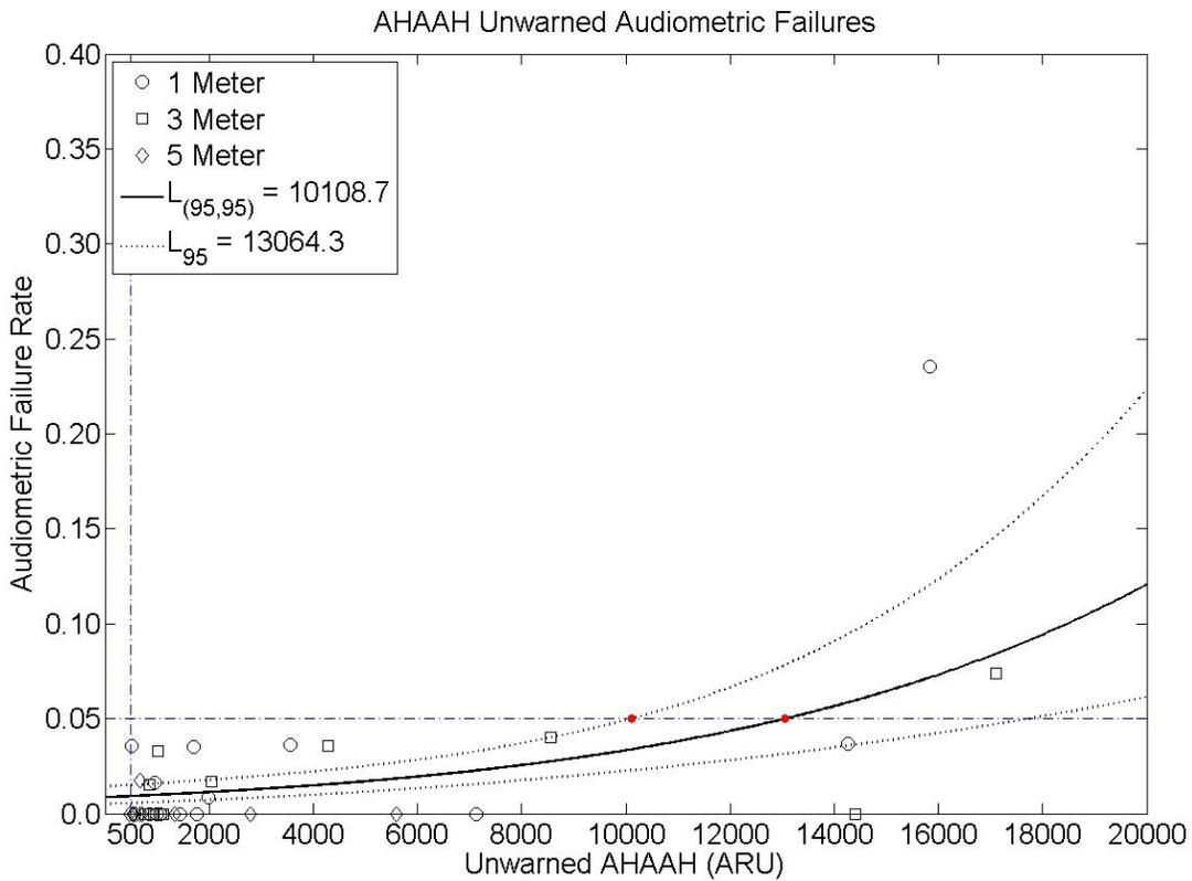
Figure 8: Evaluations of 1, 3 and 5-meter exposures using the unwarned AHA AH model using the audiometric failures. The logistic regression curve and 95% confidence intervals are shown as the solid and dotted lines. The  $L_{(95,95)}$  and  $L_{95}$  points are plotted with a solid dot symbol. The 5% failure criterion and the 500 ARU suggested damage-risk criterion are shown as horizontal and vertical dashed-dotted lines.
