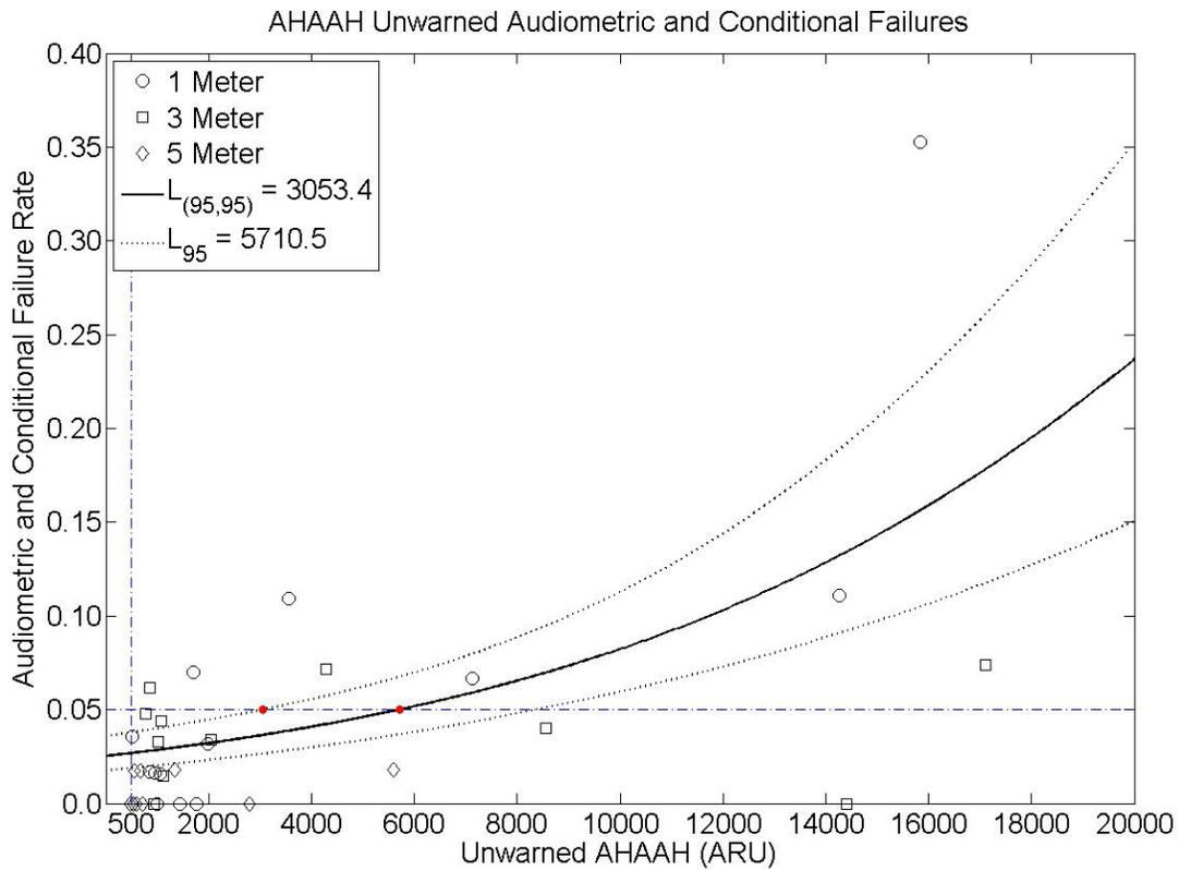
Figure 9: Evaluations of 1, 3 and 5-meter exposures using the unwarned AHA AH model using the audiometric and conditional failures. The logistic regression curve and 95% confidence intervals are shown as the solid and dotted lines. The  $L_{(95,95)}$  and  $L_{95}$  points are plotted with a solid dot symbol. The 5% failure criterion and the 500 ARU suggested damage-risk criterion are shown as horizontal and vertical dashed-dotted lines.
