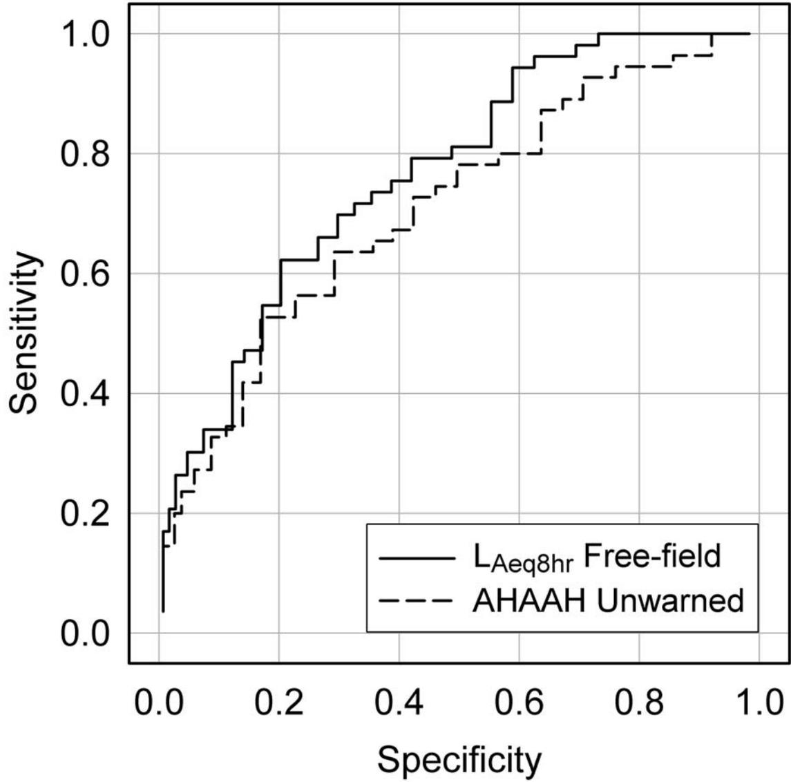
Figure 13: ROC curves for audiometric and conditional failures combined for pre-specified cells for  $L_{Aeq8hr}$  and unwarned AHA AH damage-risk criteria.
