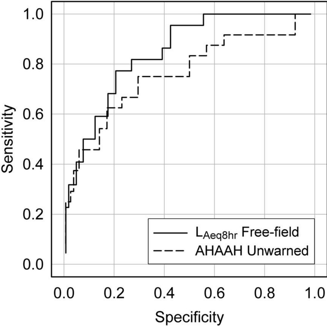
Figure 12: ROC curves for just audiometric failures for pre-specified cells for  $L_{Aeq8hr}$  and unwarned AHAH damage-risk criteria.
