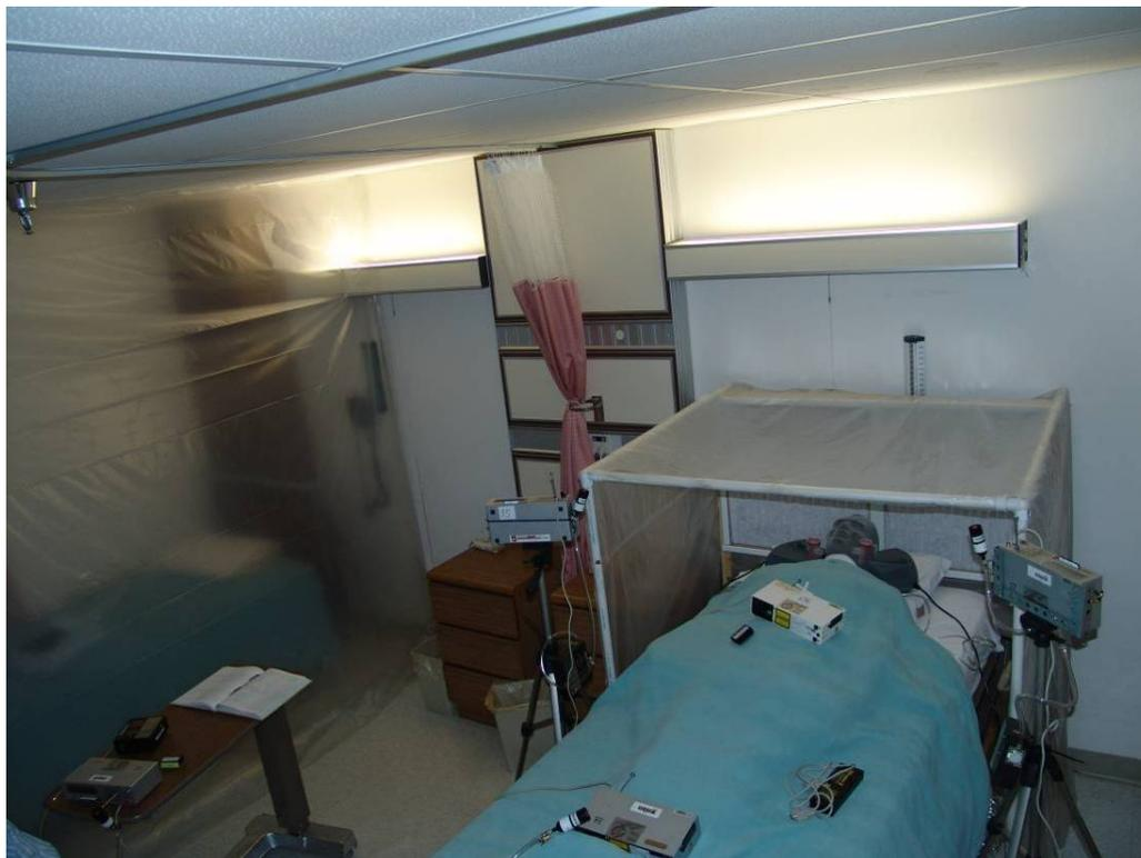
Figure 32. Photograph of ventilated headboard configuration as constructed for field research at St Joseph Memorial Hospital, in Larned, Kansas.
