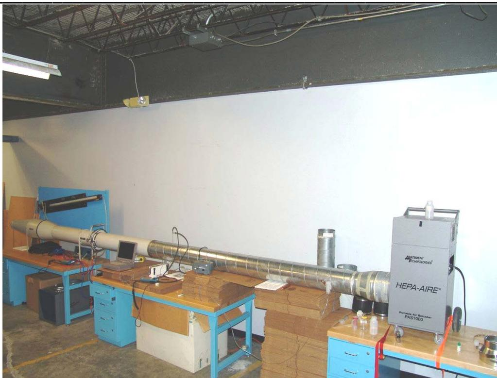
Figure 7. Schematic (7a) and photograph (7b) showing the testing platform used for development of the aerosol generation protocol.
