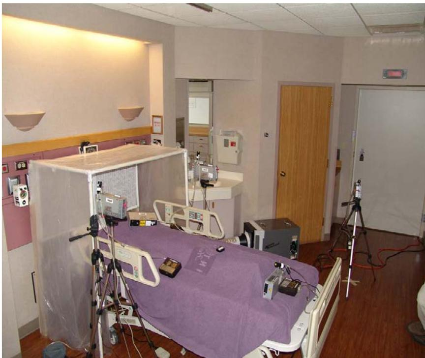
Figure 14. Photograph of ventilated headboard configuration as constructed for field research at the INTEGRIS Baptist Medical Center, in Oklahoma City, OK.
