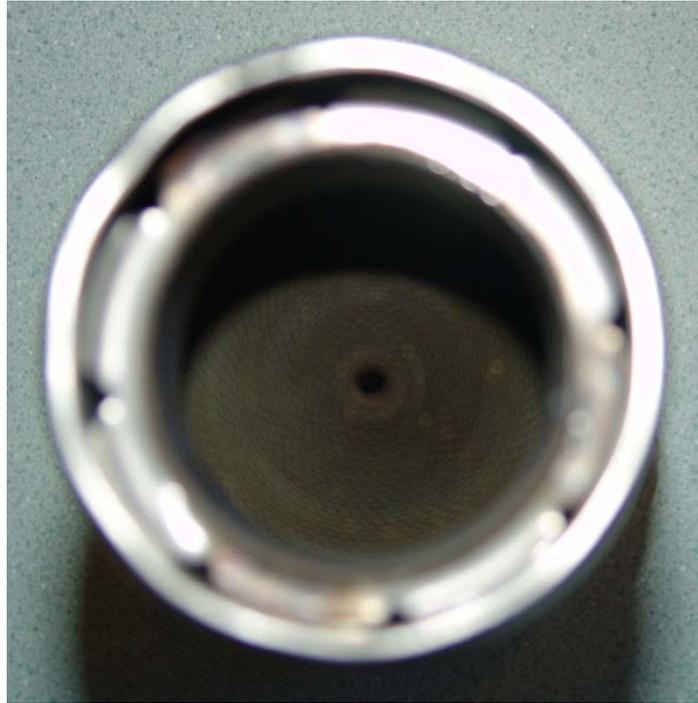
**Figure 12 - Photo of the 15 kW Kohler Old Catalytic Converter**
