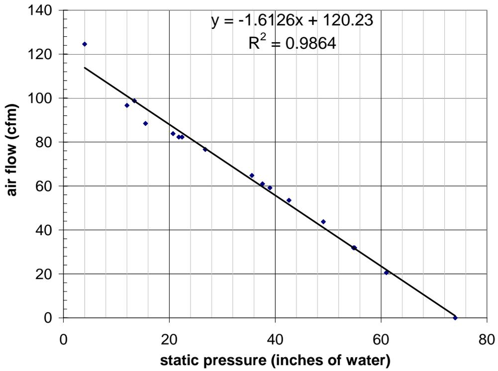
Figure 9: Fan curve for Bosch vacuum cleaner
