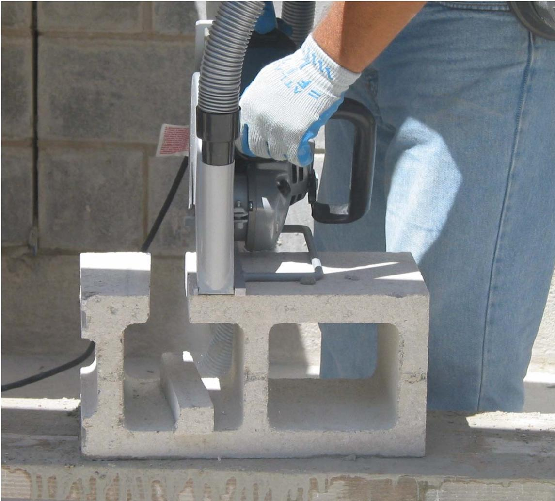
Figure 5: The Bosch cutter with shroud. Note the close contact between the shroud and block surface, essential to effective dust control.
