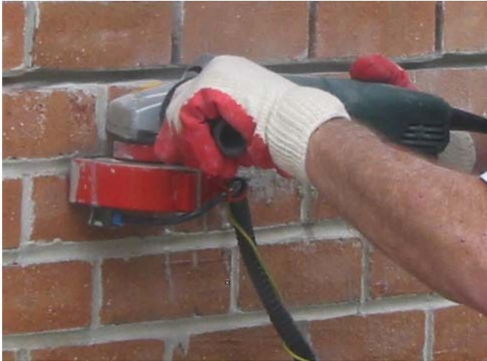
Figure 7: Grinder with Bronco control
