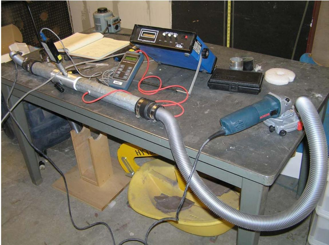
Figure 2: Experimental setting for measuring air flow and static pressure. The duct tape has not yet been applied to the flexible couplings.
