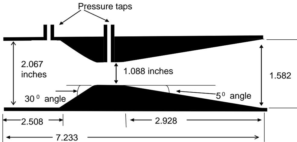
Figure 4: Description of venturi meter with dimensions measured in inches and angles from supplier's drawings. All dimensions are in inches. The venturi meter was machined from type 304 stainless steel. Wall thickness is 0.23 in. The exterior shape is a nominal schedule 40 pipe with national pipe threads on the ends.
