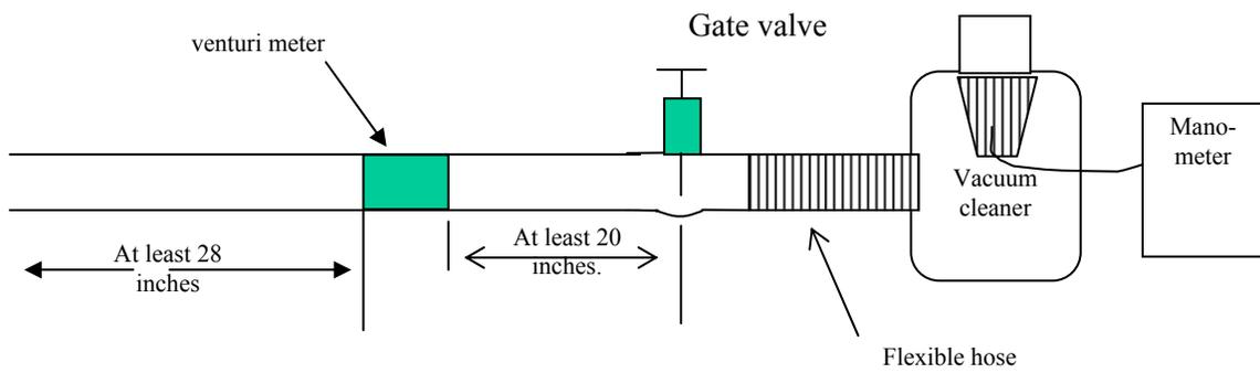
Figure 3: Experimental measurement of pressure loss as a function of airflow rate for commercially available vacuum cleaners. The pipes used in this study are 2 inch diameter schedule 40 PVC pipe. The vacuum cleaner static pressure is measured between the final filter and the inlet to the vacuum cleaner motor.
