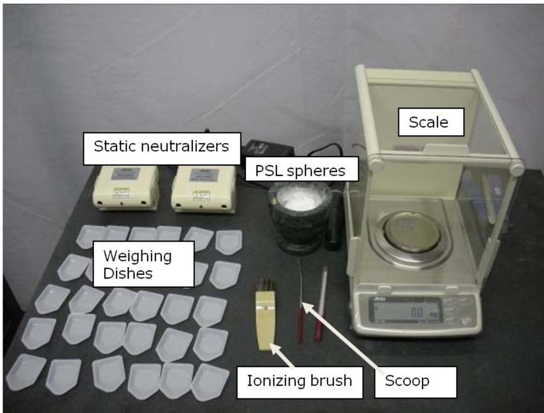
**Figure 3: Set up for the weighing process**
