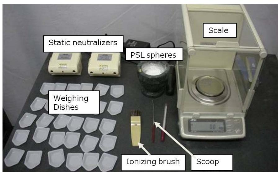
**Figure 3: Set up for the weighing process**
