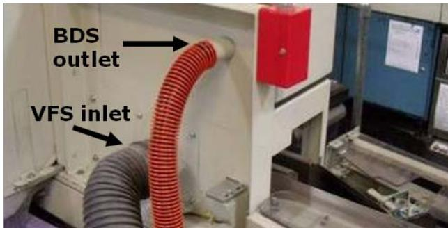
**Figure 17: BDS outlet and VFS inlet locations on the flats extractor**
