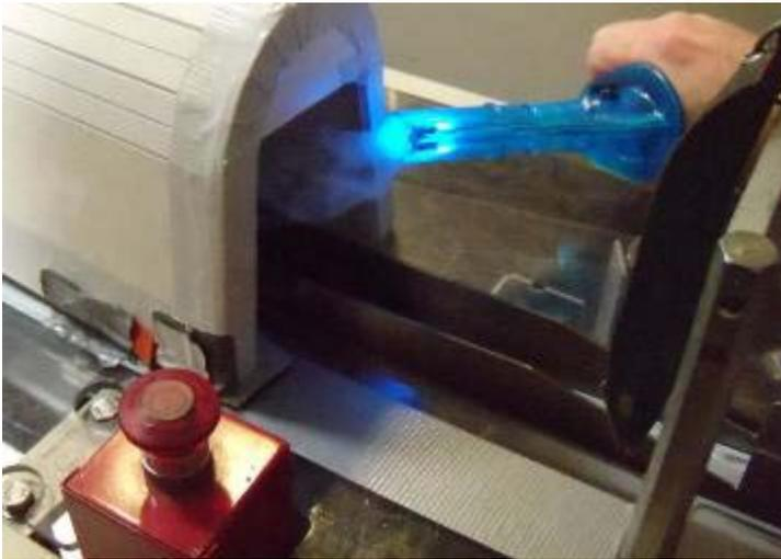
**Figure 26: Smoke entering the influence of the hood extension on the prototype AFCS 200 machine**
