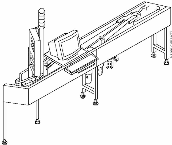
**Figure 3. Singulator Area of the AFCS.**
