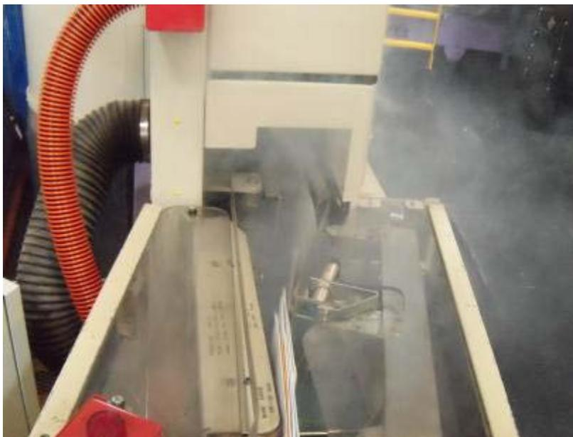
**Figure 20: Smoke escaping from the enclosure adjacent to the flats extractor**
