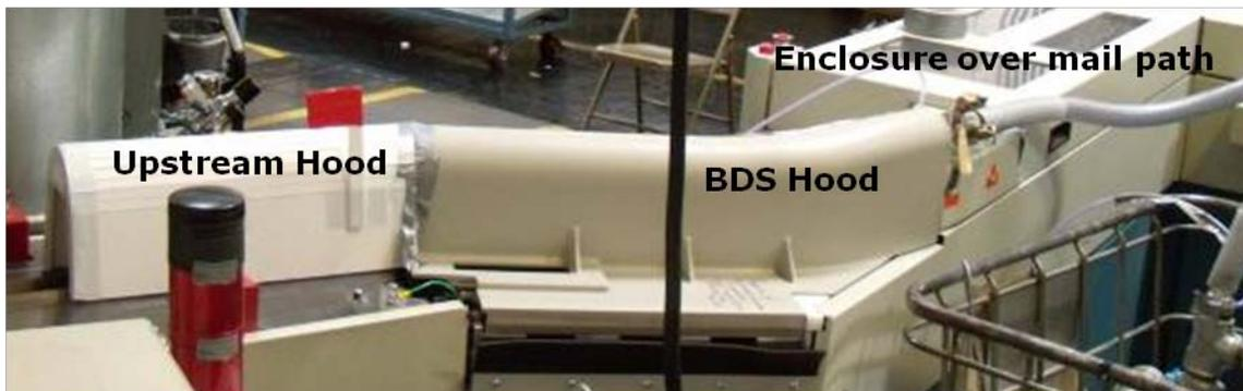
**Figure 5: BDS Hood on the Prototype AFCS 200**
