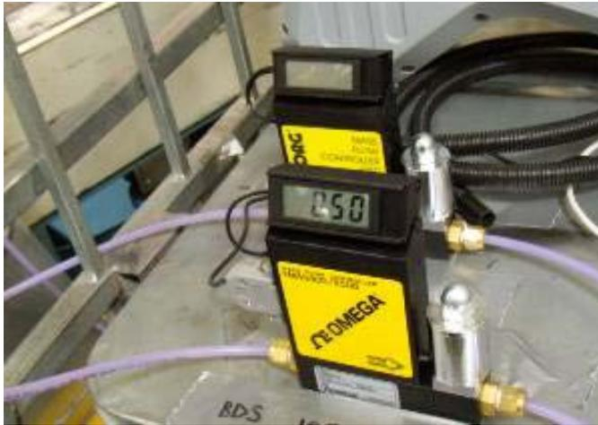
**Figure 12: Aalborg and Omega Mass Flow Controllers**
