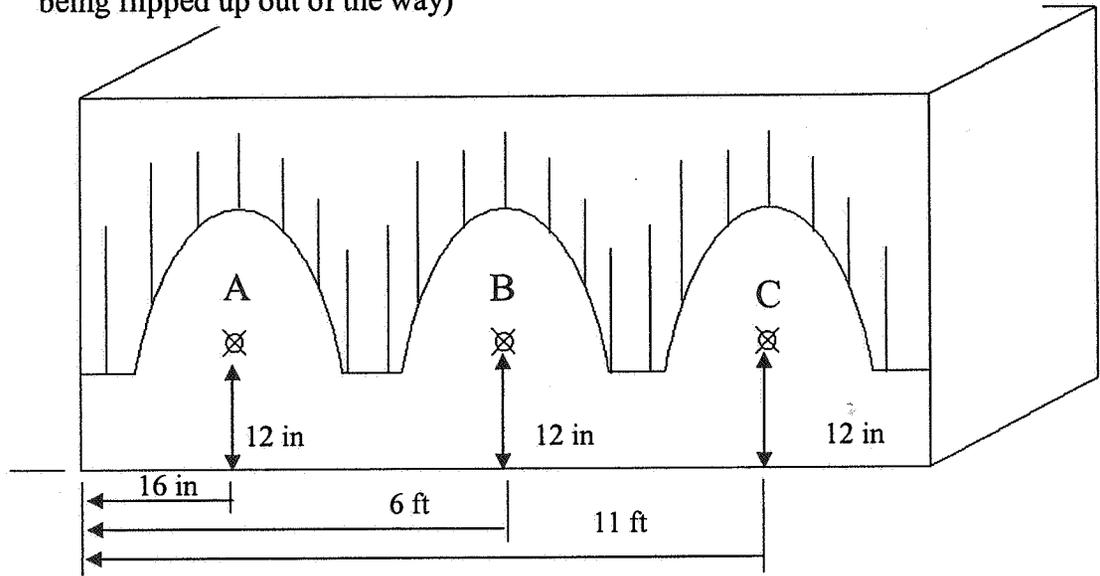
Figure 3: Location of testing points for unmodified curtain (configurations C & D)
