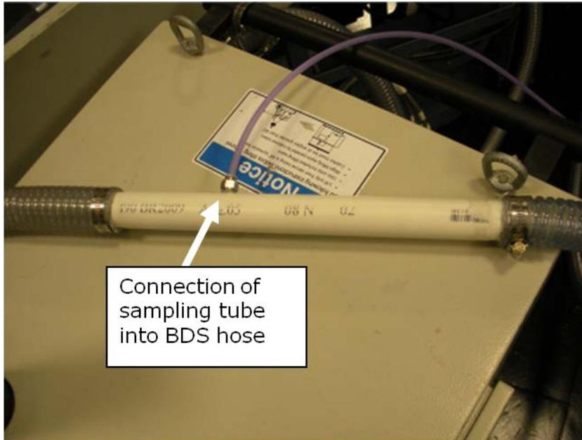
**Figure 5: Connection of sampling tube to the BDS hose**
