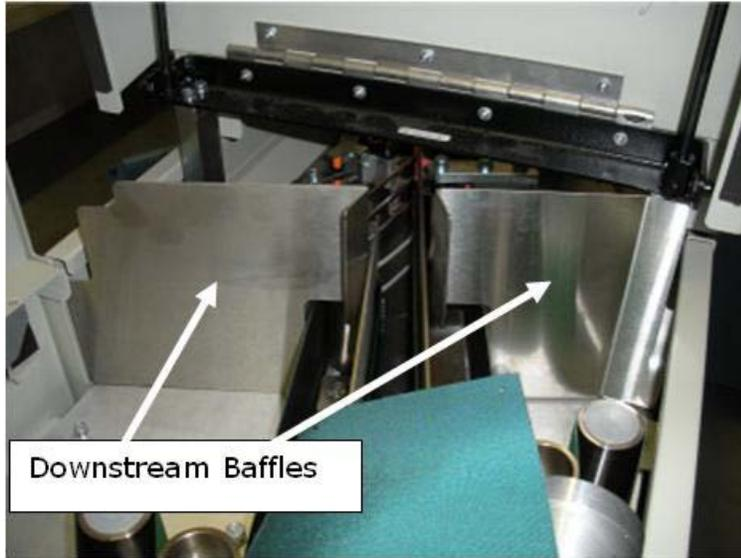
**Figure 1: Downstream baffle near the first cover**
