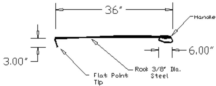
Figure 13. Sorting Parts Hook
