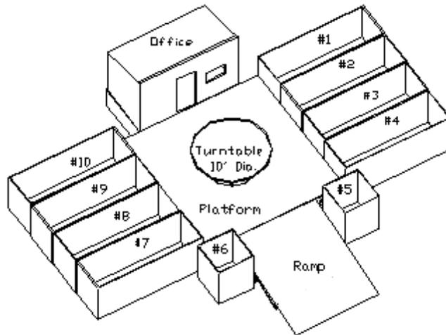
Figure 12. Elevated Rotating Sorting Table
