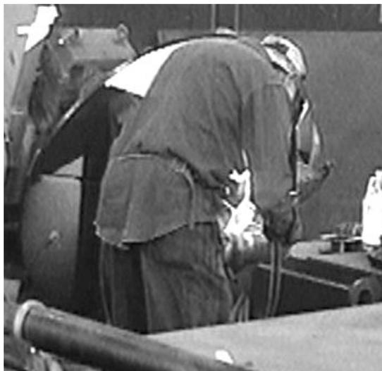
Figure 7. Welder Welding Piece in Flexed Posture Despite Positioner
