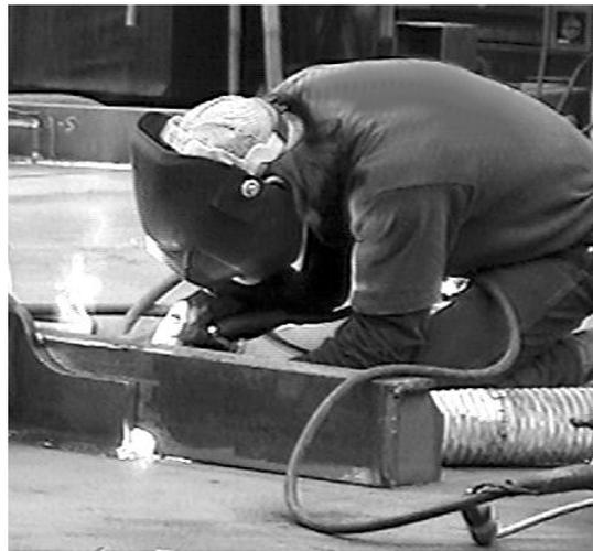
Figure 14. Panel Line Welder Wire Welding
