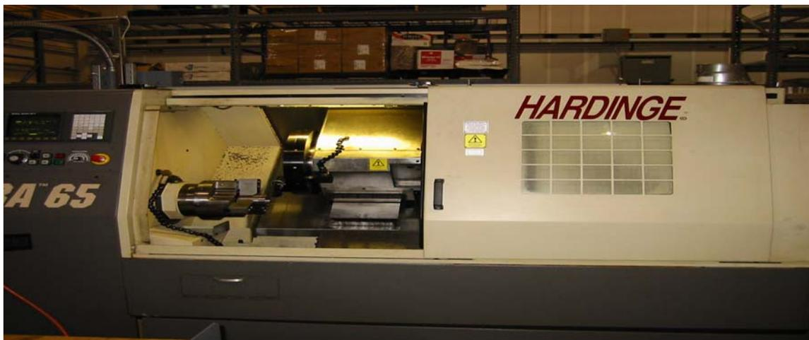
**Figure 4. Hardinge Cobra 65, machining center for turning tests.**
