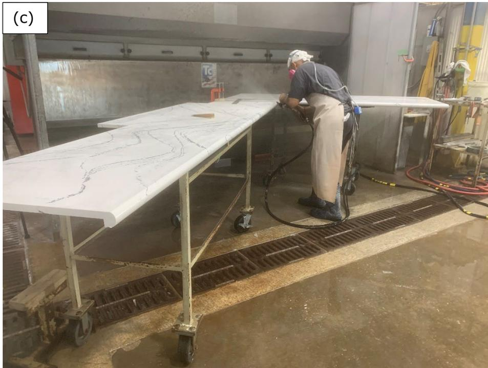
**Figure 3 – (a) Two workers working in front of a MB60 water wall dust extractor (Unit 1 in Figure 2a) in the final grinding/polishing process in Setting 1; (b) a worker conducting the grinding task in front of a MB60 water wall dust extractor in Setting 2; (c) a worker conducting the grinding task in front of a MB40 water wall dust extractor in Setting 3. Photos by NIOSH.**
