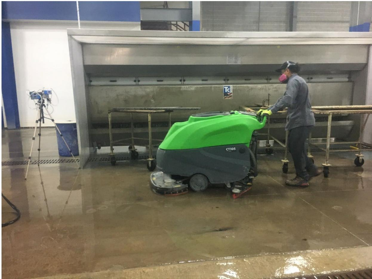
**Figure 4 – A worker operating a CT105 wet scrubber to clean the floor of the fabrication area. Photo by NIOSH.**
