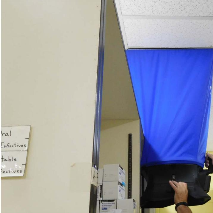
Figure 5. TSI Accubalance<sup>®</sup> Plus Air Capture Hood (Photo Credit: NIOSH)
