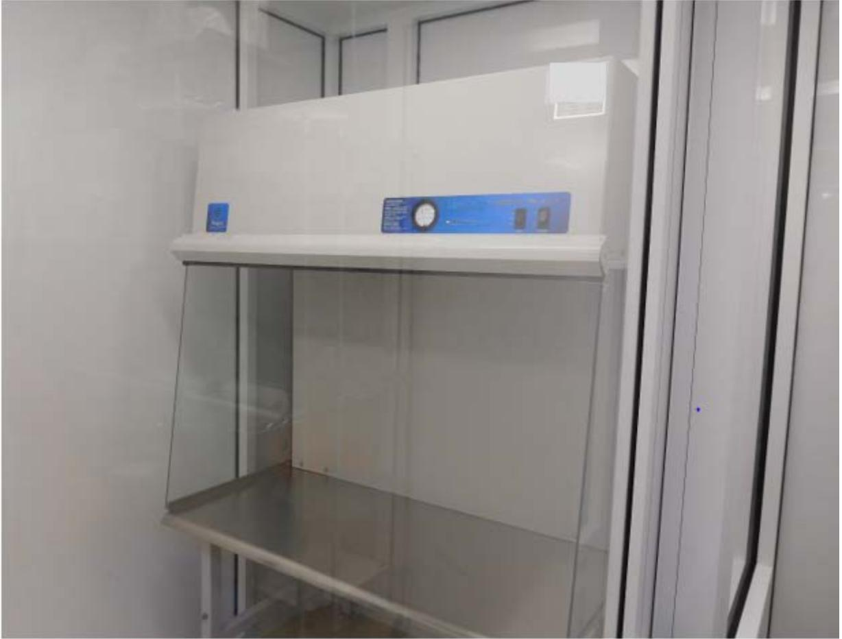
Figure 1. Labconco Laminar Air Flow Work Station (Photo Credit: NIOSH)
