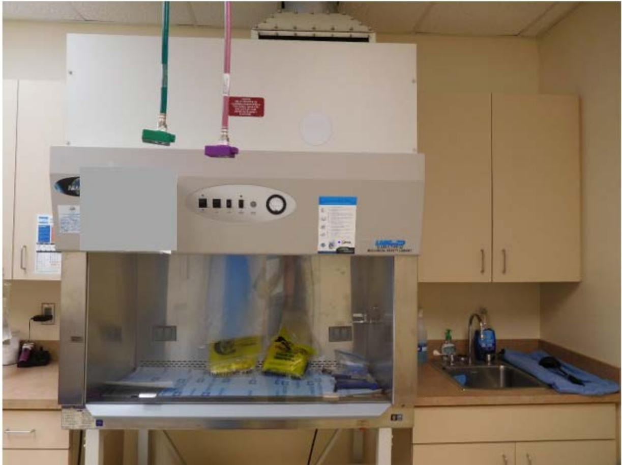
Figure 1. BSC, Nuair Labgard Class II, Type A2 (Photo Credit: NIOSH)
