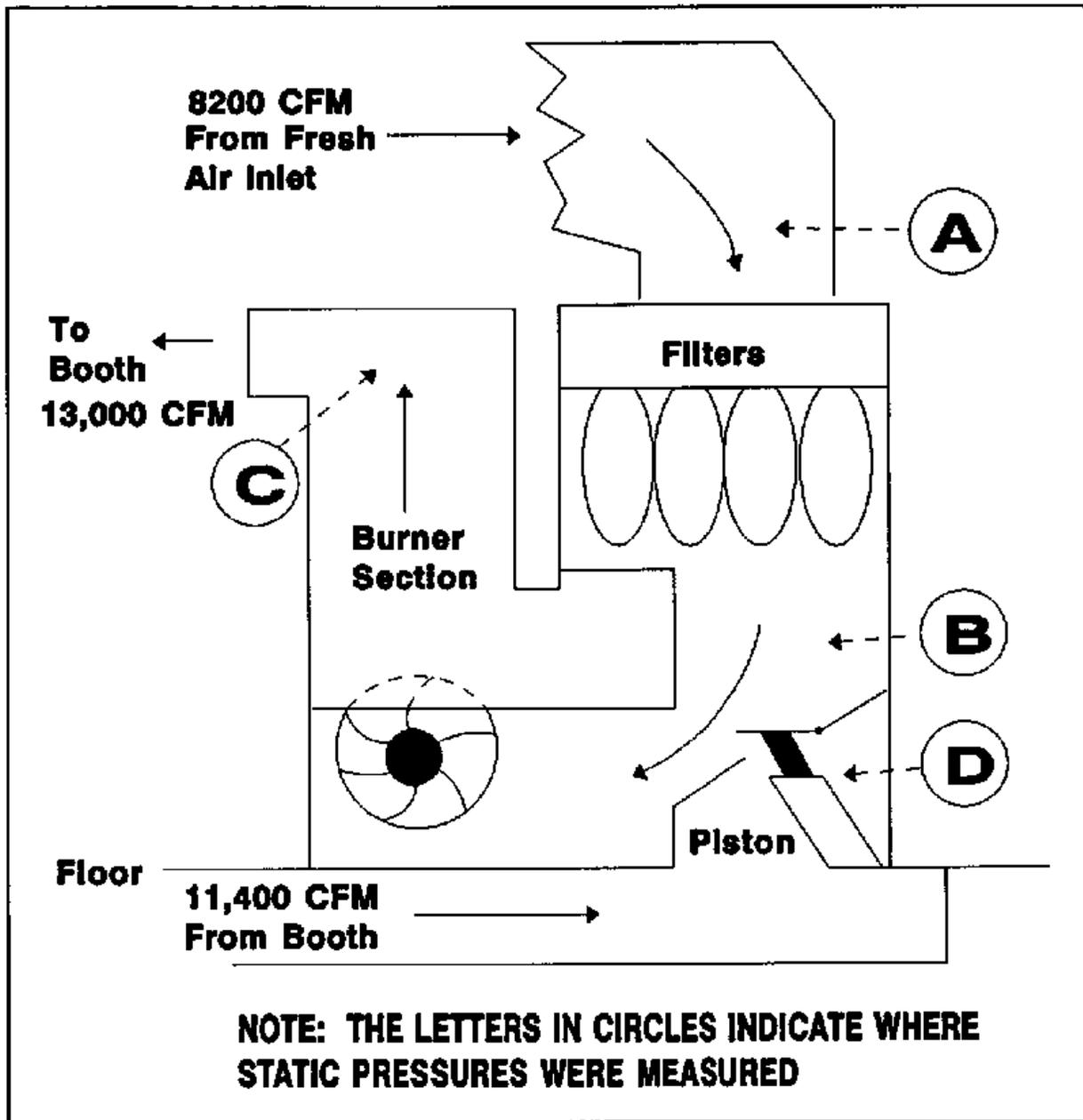
Figure 5 Side view of ventilation system for the spray painting booth
