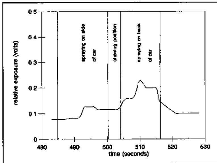
Figure 9 Relative exposure while spray painting car at the vehicle preparation station
