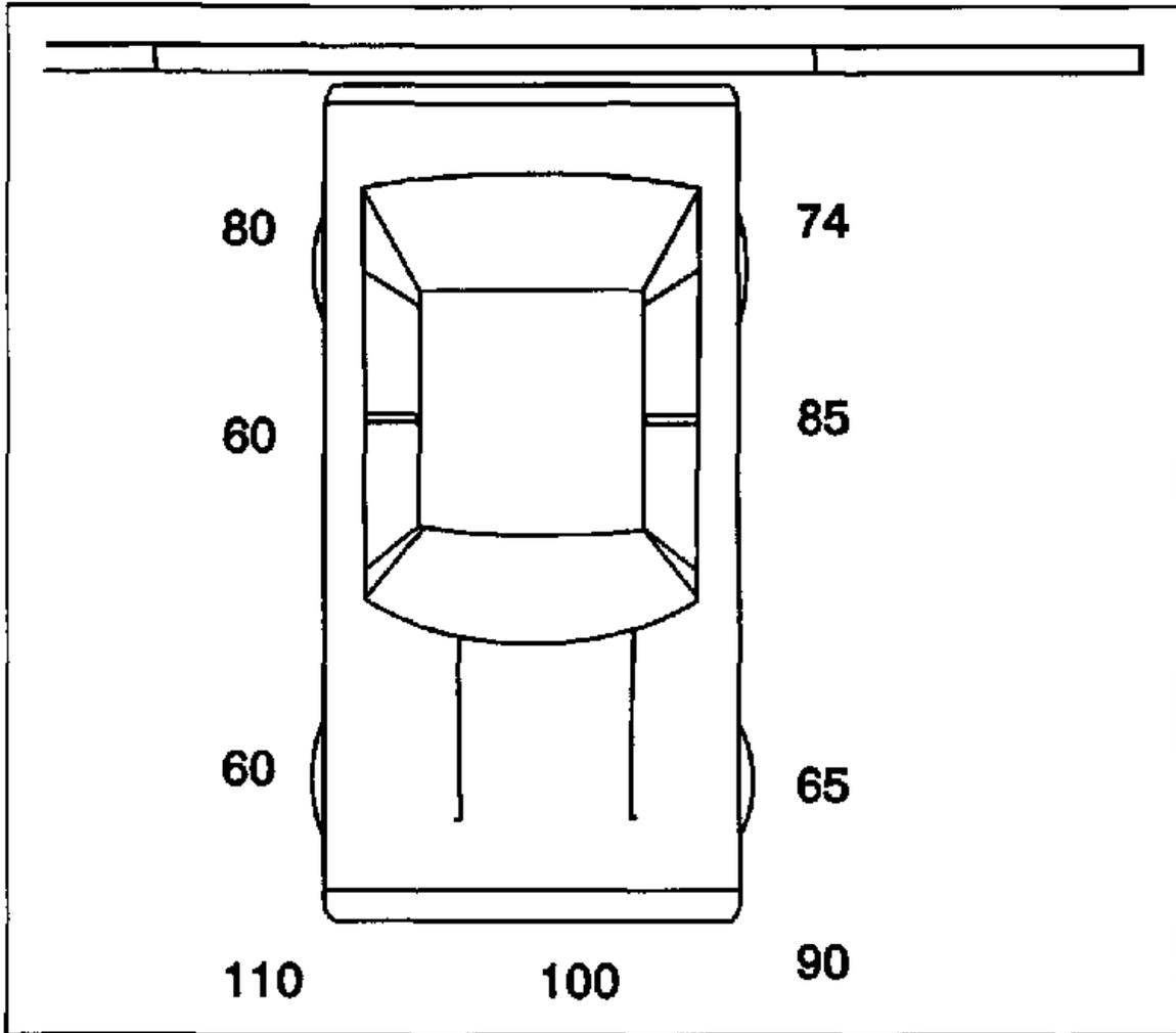
Figure 6 Air velocity (feet per minute) around car at a height of 3 feet and a distance of 1.5 feet from the car
