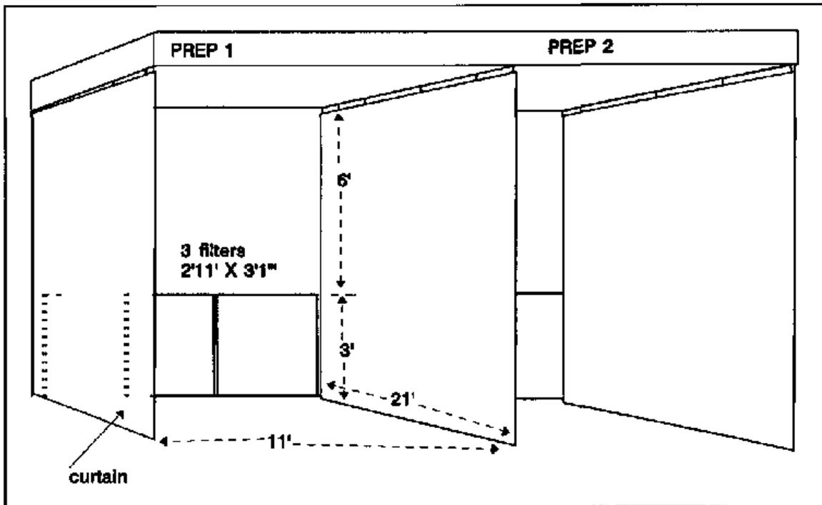
Figure 2 Schematic illustration of vehicle preparation station
