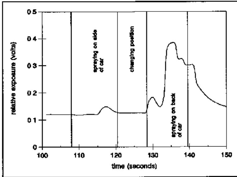
Figure 8 Relative exposure while spray painting car at the vehicle preparation station
