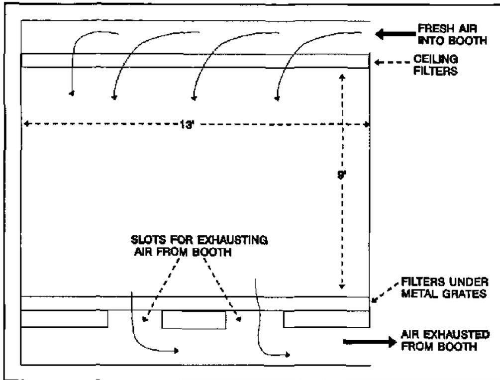
Figure 3 Schematic of spray painting booth
