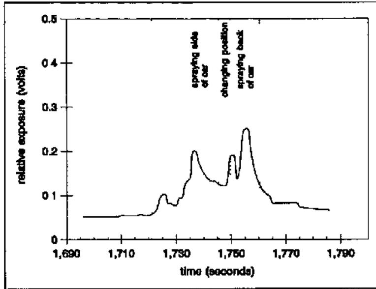
Figure 10 Relative exposure while spray painting car at the vehicle preparation station
