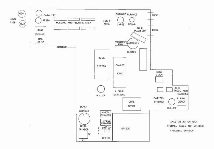
Figure 1. Schematic layout - General Foundry Company.
