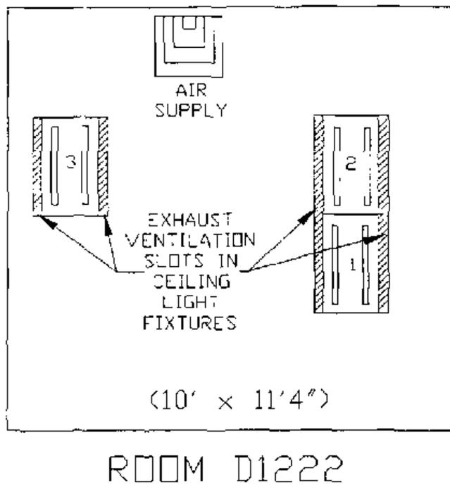
Figure 5 A Plan View of the Ventilation Sampling Areas and Room Layout
