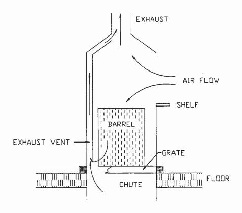
Figure 5. Bag dump station - side view.
