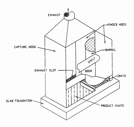
Figure 7. Bag dump station - isometric view.
