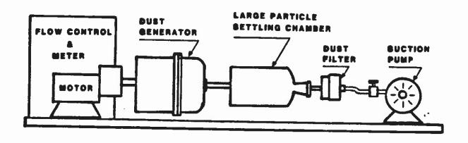
Figure 8. Heubach Dust Measurement Appliance.
