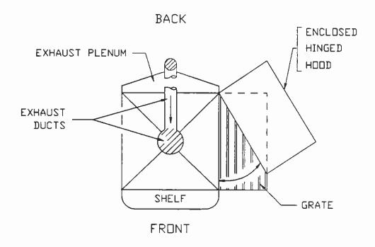
Figure 6. Bag dump station - top view.
